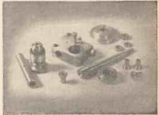
Fig. 4 (Below).—Components of toolpost drilling and milling spindle, including collets and drill chuck adaptor.
