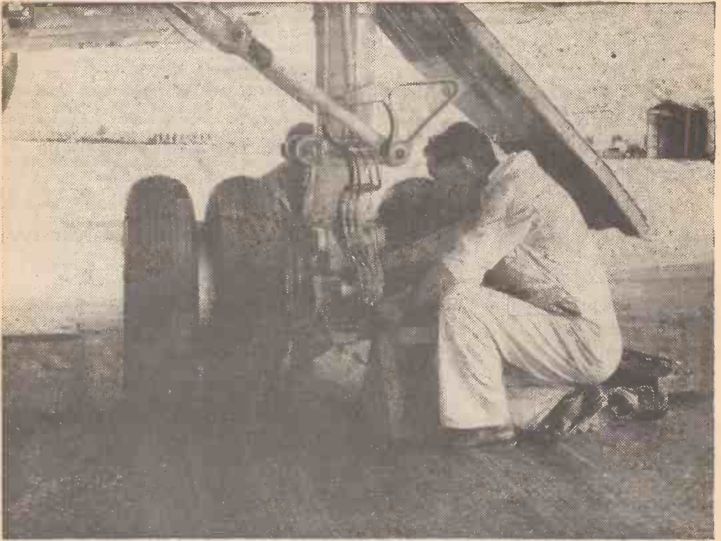
Photograph shows close-up of undercarriage wheel arrangement on the main oleo, also main retracting arm and wheel well cover. The mechanic servicing the undercarriage gives some idea of the size.
