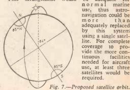
be adequate for normal marine use, thus astronavigation could be more than adequately replaced this system using a single satellite. For complete coverage to pro-vide the more continuous facilities needed for aircraft use, at least three satellites would be required.
