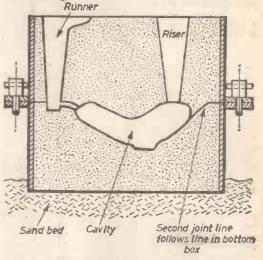
Fig. 7.—Moulding irregular shaped articles.
