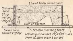
Fig. 1.—First stage in the preparation of a mould,
