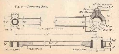
in Fig. 64. Note that it projects through  $\frac{3}{44}$  in, and forms a distance-piece between the coupling-rod boss and the big-end. The projection which represents the full-size oil box is drilled No. 40, tapped  $\frac{1}{4}$  in. or 5B.A. and furnished with a hexagon-headed brass screw, drilled through No. 55, the head being counterbored  $\frac{3}{32}$  in. This screw runs right into the big-end bush as shown in Fig. 64.
