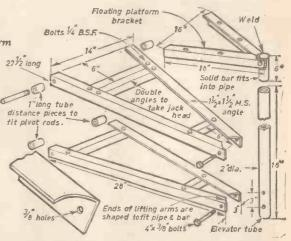
The elevator tube is an 18in. length of 2in. dia. pipe drilled with \$\frac{1}{8}\$in. holes at 3in. centres to accommodate the cross bolts of the lifting arms. With the jack in position, the tube should rise and fall vertically from floor level to maximum height. Adjust the screw neck of the jack piston to give contact with the angles of the upper arm when the piston is at lowest stroke.
