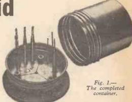
With regard to construction, the holes to carry the drills are made by the drills themselves and, in this way, they also serve to identify the drill sizes. The holes for taps should be drilled to the shank diameter (taps should never be nested by their threads). Fortunately, no identification problem arises with taps, as the sizes are always marked on the shanks.
