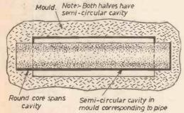
Fig. 6.—Plan of the mould for the pipe shown in Fig. 5.
