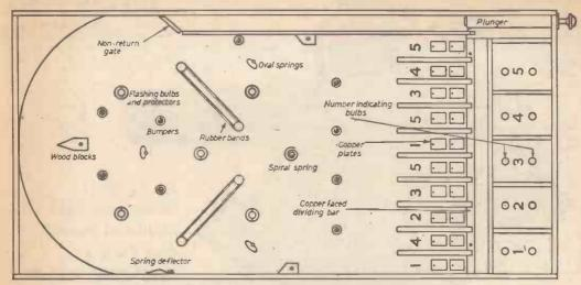
Fig. 7.—Plan of the lay-out of hazards, etc.
