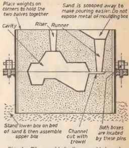
Fig. 4.—The mould finally assembled ready for pouring.
