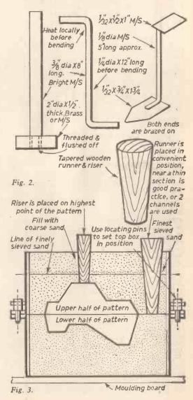
then carefully set the lower box on a bed of moulding sand. Locate the top member and you are ready for the pouring. Fig. 4 illustrates the mould assembled on the foundry floor ready for the running of the metal.
