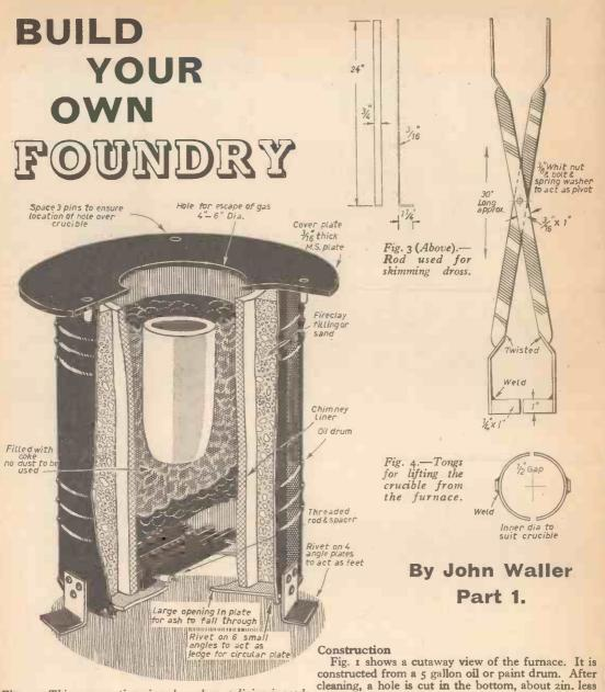
Fig. 1.—This cross section view shows how a lining is made and the method adopted for holding the lower fire bar plate.
