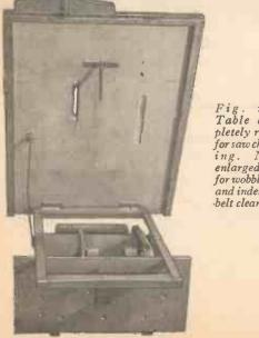
Fig. 2.-Table completely raised for saw changing. Note enlarged hole for wobble saw and indent for .belt clearance.
