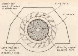
Fig. 3.—Conventional Induction motor showing armature, field coils, and method of rotation.
