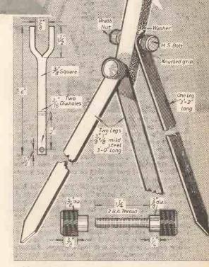
Measurements and constructional details of the rest.
