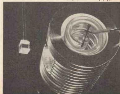
Glowing with absorbed light is a synthetic ruby crystal (left). A light source (right) pours "random" waves of light into the ruby.
