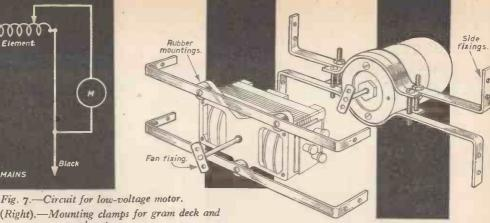
Fig. 8. (Right).—Mounting clamps for gram deck and round motors.
