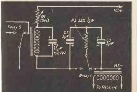
Fig. 12.—Ratio sensitive circuit.
