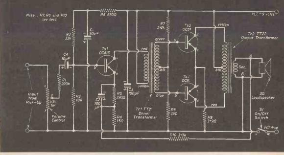
Fig. 5.—Amplifier circuit diagram. Experienced readers may prefer to use this instead of the wiring diagram.
