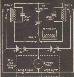
Fig. 11.—Steering motor circuit.
