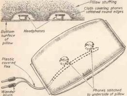
Fig. 1.—Installing the earphones.
