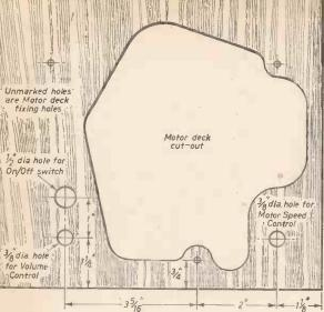
Fig. 3.—The cutaway portion and drilling positions of the motor board.
