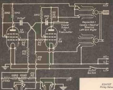
Keyswitch 2 Increase/Reduce Fig. 15.—The multivibrator control
