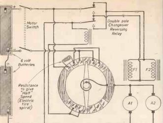
Fig. 9.—Connecting the speed control unit to batteries and motors. F = field and A = armatures.
