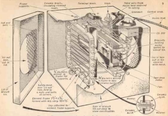
Fig. 4.-Cutaway perspective view of the complete heater.
