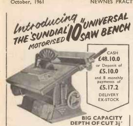
Allows a range of operations far wider than other Sawbenches. Precision built, 20" × 21" precision machined saw table, complete with table mitre slide, and calibrated tilt to 45 deg. Rip fence with a special micro fine adjustment, also supplied one mitre fence, 10" rip tooth blade. Mounted on a well designed bench stand; motorised, 3 phase electric motor, press button starter. 10 ft. rubber lead fitted for immediate use. Write for leaflet giving details of accessories.
