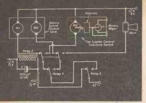
—the lamp control servo motor operates and switches on and off the vehicle lights in sequence.
