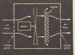
Motor A small tape recorder motor (induction type) is used in the prototype shown; further details are given in the text. Some electric gram. motors will suit and, with alterations to the circuit, surplus 24V. types will do.
