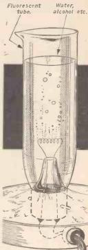
Fig. 71.—A simple immersion heater for non-corrosive fluids. Dowels.
