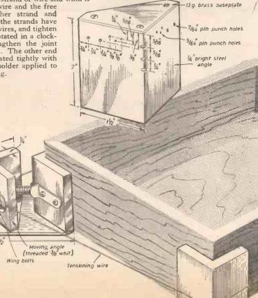
Fig. 2.—Dimensions and general details of the cramp.
