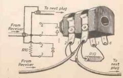
Inserting jack plug closes contacts 1 and 4, and opens 2 & 3 Fig. 159.—How the system of Fig. 156 is wired up in a practical manner. See also Fig. 154. (Left) Theoretical wiring plan.
