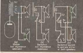
Fig. 157.—Various extension speaker systems. Tr1 is the transistor or value output transformer. Loudspeakers 1, 3 and 5 are the original ones, 2, 4 and 6 are extensions. S2 and S3 are ganged.
