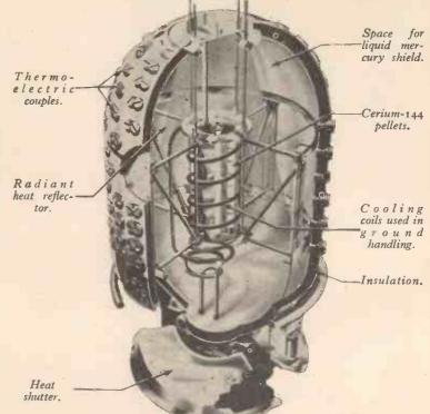
A cutaway drawing of the SNAP 1-A atomic generator shows the outer thermocouple studded metal container and the device's inner construction. During the ground-handling prior to launching, the hollow interior of SNAP 1-A can be filled with liquid mercury, which acts as a radiation shield. The mercury would be drained out moments before lift-off to reduce weight.
