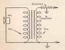
Fig. 4.—The transformer connections.
