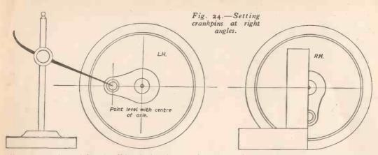
adjust the wheels until they do. When both rods are on, and the wheels turn freely without binding anywhere, the rest of the wheels can be pressed righthome.
