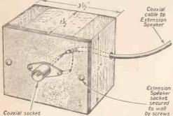
Fig. 155.—A very simple form of extension speaker socket fitted in a box for screwing to the wall.
