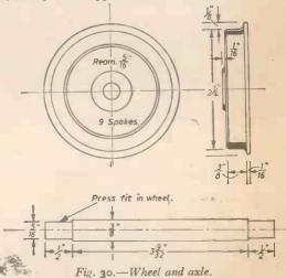
from §in. round mild or silver-steel rod, to the dimensions shown in Fig. 30. Oil ducts are not required in the pony axle, as you can poke the spout of an oil feeder between the wheel spokes, and put a drop down the oil holes on top of the axleboxes.
