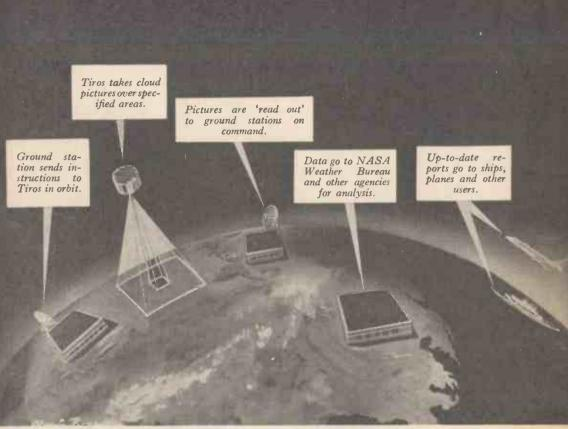
The major orbital and ground elements of the Tiros II television-infrared weather observation system.
