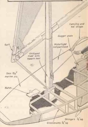
Fig. 1.—Cutaway perspective view showing general construction and rigging details. Fig. 2.—Centre-board box details. This will be described next month.
