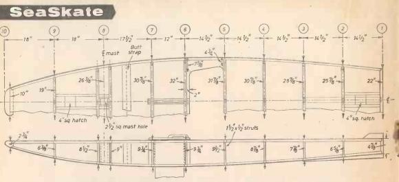
Fig. 5.—Plan and side elevation showing all framing, centre-board box and mast box.
