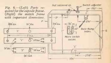
capsule to expand and operate the microswitch, changing over the lamp circuit.
