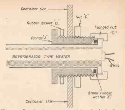
Fig. 4.—Surplus heater mounted in plumber's flange fitting.
