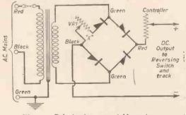
Fig. 2.-Substituting a variable resistor.
