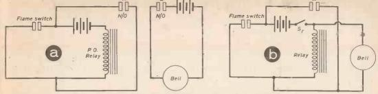
Fig. 141.—(a) A simple circuit without test or re-set provision, using separate batteries for relay and bell. (b) A simple circuit using one battery, with provisions for re-set but not testing.
