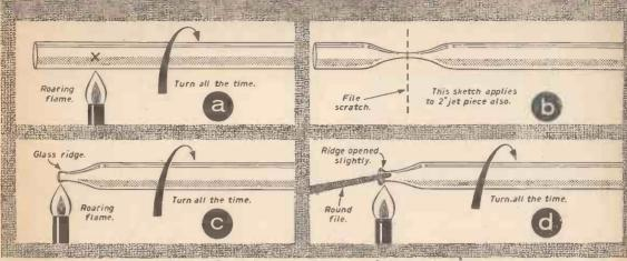
Fig. 53.-Stages in forming the lower end of a burette.
