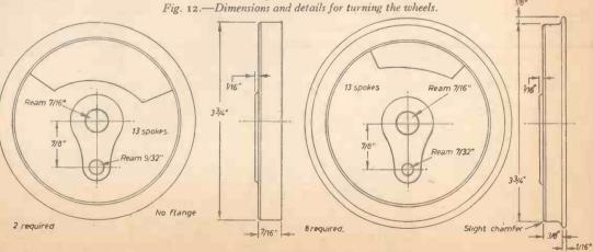
central. Clamp the jig to the wheel boss, and drill the boss  $\frac{1}{3}$  in. using the hole in the jig to guide the drill. After drilling all ten, put a  $\frac{1}{32}$  in. parallel reamer through all the holes in the flanged wheels. Those in the driving wheels (flat treads) are opened out with a  $\frac{1}{34}$  in. drill and reamed  $\frac{9}{32}$  in. Bigger crankpins are needed to take the driving stresses.
