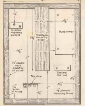
Fig. 3.—Rear mounting board showing positions of various components.
