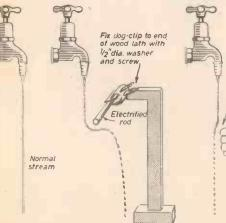
Fig. 1.—Adjusting the faucet and deflecting water.
