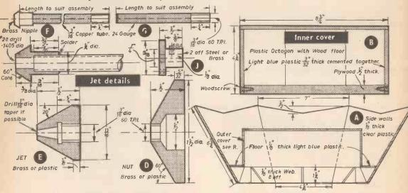
Fig. 3.—Details for making the jet.
