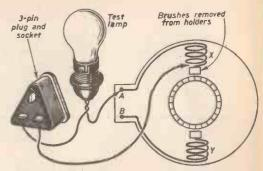
Fig. 4.—Testing for an open-circuited field coil in a series motor.
