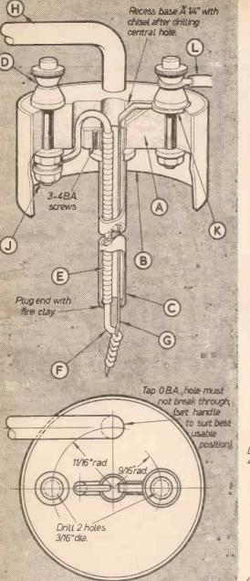
Fig. 1.—Pyrometer assembly. A-base; B-cover; C-tube; D-terminal; E-insulating beads; F-24G Nichrome wire; G-copper strip; H-handle; J-clamping nut.
