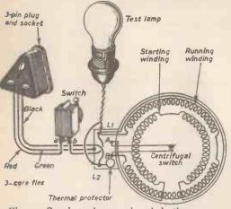
Fig. 1.—Supply testing a 1-phase induction motor.
