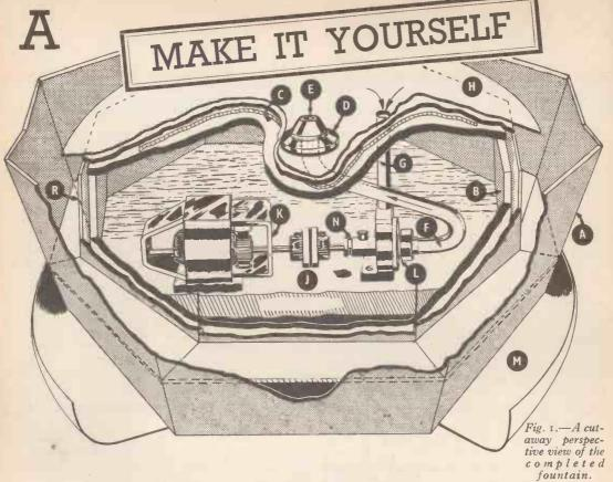
THE design consists basically of a small pump, driven by a motor which, though arrangements can be made to run it off the mains, the makers, Stuart Turner Ltd., Henley on Thames, Surrey, claim will operate from ordinary torch batteries. Described as an S.T. electric motor, it weighs 6 oz. and costs 25s. This is mounted in a plastic bowl. The making of the octagonal bowl (Figs. 1 and 4)
