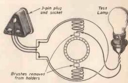
Fig. 6.—Testing a series model for short circuited armature.
