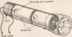
Fig. 2.—Section of a torch modified for testing. Fig. 3. (Below)-Testing for an open circuit in a series motor.
