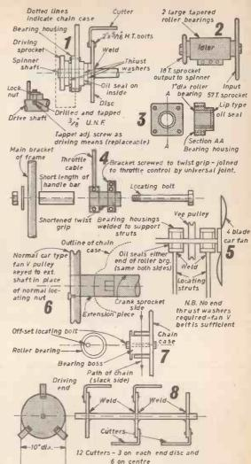
Fig. 1.—Spinner end thrust and driving device. Fig. 2— The idler. Fig. 3.—Spinner end bearings. Fig. 4.— Throttle twist grip installation. Fig. 5.—The fan drive. Fig. 6.—Fan drive pulley from crank shaft. Fig. 7.— Spinner drive chain adjustment. Fig. 8.—Spinner discs and cutters.
