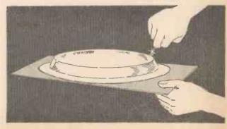
Having now described the generation and testing of a static charge, we can also proceed to experiment. Assuming you have "excited" the sheet and placed the baking tin in position, put a little pile of puffed rice or oats, or chips of elder pith on the top of the tin. On lifting the sheet the pile will disintegrate and the puffed oats will fly up into the air. I once tried a pile of dry flour and this flowed into the air in a steady stream like a snowstorm.
