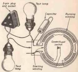
Fig. 5.—Testing for an earth fault on a capacitor start induction motor.
