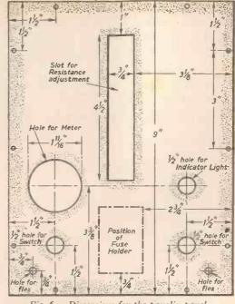
Fig. 6.—Dimensions for the paxolin panel.
