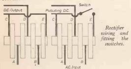
transformer is taken to terminal A and B. The D.C. output is taken from the terminals C, D and E, D being positive and C and E being negative. As C and E are only used on alternate half cycles, they are coupled together. The effect of breaking this coupling is to cut off the power for half of every cycle giving pulse power. The switch should be fitted as shown above right.—S. R. Broadfoot (Dunstable).
