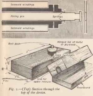
Fig. 3.—(Below) Box for the device and the control box.
