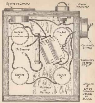
Fig. 3.—Point to point wiring diagram.
