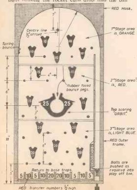
trap at the bottom end of the table. The trap is made entirely of  $\frac{1}{4}$  in. ply with a back measuring in. × 16 $\frac{3}{4}$  in. and the legs from pieces in. × 2in. End divisions are spaced at  $\frac{1}{4}$  in. but those between are all at 1 $\frac{3}{4}$  in. centres. Paint the trap yellow (Fig. 7).
