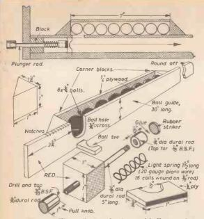
Fig. 2.—The striker mechanism and ball magazine.
