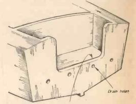
Floor of well low enough to provide enough space for clamps of engine on transom. Sea-going transom with self-draining well
