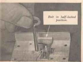
Scribe a mark in line with the bottom of the slot in the bolt and remove the surplus metal to the thickness of the bolt
