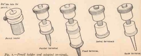
stood that the lower portions of all these terminals are tight fits and that only the tops revolve by hand pressure on the milled edges; the bar or bars lie between the terminal heads and bases and are locked or loosened as required.
