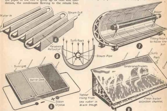
Fig. 4.—Solar collector for steam generation. Fig. 5.—Details of operation of reflectors. Fig. 6.—A solar battery. Fig. 7.—Giant solar powered steam generator. Fig. 8.—Solar still to make fresh water from salt water.
