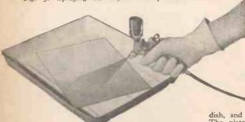
The silvering solution should be treated with hydrochloric acid to precipitate any excess silver. If this is not done, the solution will in time deposit a very delicate explosive compound which can prove exceedingly dangerous when handled.
