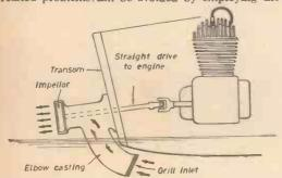
principle illustrated above. Water is drawn from beneath the engine and thrust out at an angle of 90 deg. I have a proprietary engine working on this principle. A similar type is available using a horizontal impeller and a vertical drive shaft, so that
