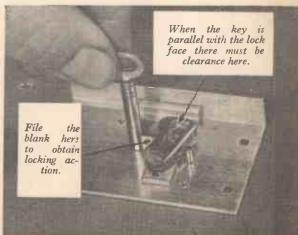
Fig. 7 (Above).—Cutting the blank to the levers.
