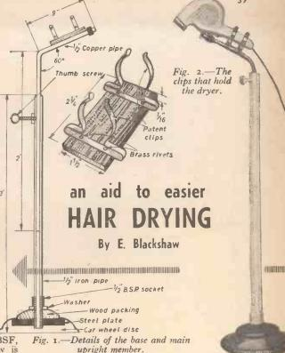
Two Terry Spring clips No. 80/5 are riveted to a piece of brass or copper plate using the existing two holes in each clip. See Fig. 2. The plate is then brazed or bronze welded longitudinally by a fillet to the copper tube. The base is black enamelled and the upright smoothed down and enamelled cream, the copper being polished and left unpainted.
