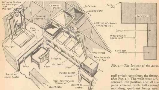
described these are for a safelight, dish heater, enlarger, enlarger/printer and a spare for fan or radio, etc.
