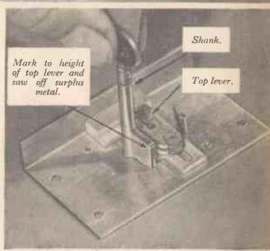
Fig. 5.—Marking the length of the blank.
