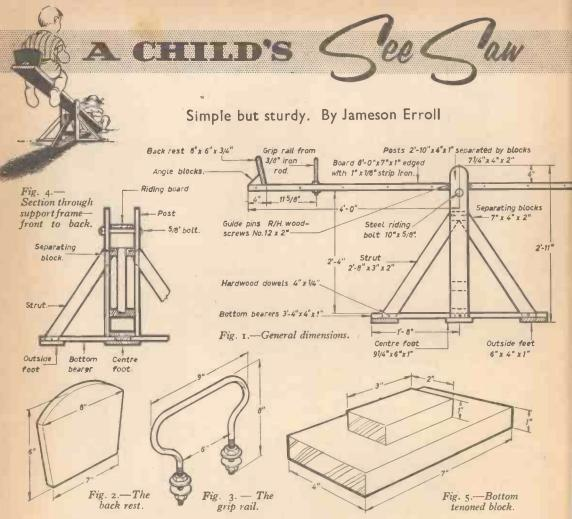
HE see-saw consists of a riding board mounted on a strutted frame. Good quality deal may be used. The board is 8ft. long, 7in. wide and 1in. thick and is strengthened by screwing in. × kin. strip iron along both edges; the screws should be iin. No. 8's. Two back rests (see Fig. 2) are screwed in position from the underside of the board, their bottom edges being bevelled to the necessary angle. They are further supported by two angle blocks to each rest; the slope is approximately 100 deg.
