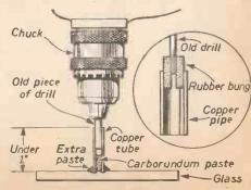
the cut. Drilling is shown in progress in Fig. 13.
