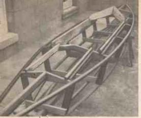
are cut to shape next. Make the splay-cut to the top and bottom first. Hold the blocks against the spine and the ridge-strip (which you have already fixed) to mark them for this. Next notch the spine and top ridge strip into the blocks. Hold the blocks loosely between spine and ridge strips and mark the sides of the blocks for rough shaping. After this has been done fix them in place. The top side strips are chamfered off and fixed to the blocks; Photo No. 5 shows this construction.
