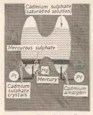
Fig. 3.— The cadmium cell.
