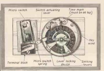
Fig. 41.—Another reconditioned timeswitch suitable for use in the home.
