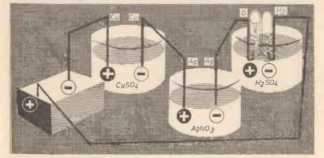
Fig. 1.—The basic principles of electrolysis.
