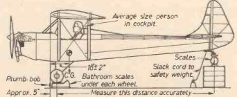
Fig. 82.—Completed aircraft set up in the rigging position on scales showing the position of the centre of gravity.
