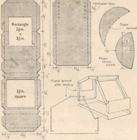
Fig. 4 .- How to mark out and assemble the frame and base sections and form the finger recesses.
