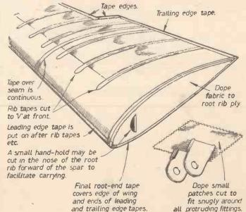
Fig. 78.—Taping operations.
