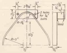
Fig. 28.—Chain guard detail for Clinton engine. Make from  $\frac{1}{2}$  in. thick or 10 gauge M|S plate. The chain guard for the J.A.P. engine is similar.
