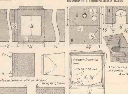
Fig. 5.-Slide and diffuser holder, lampholder and switch plate and lens securing frame.
