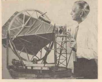
Fig. 1.—A model of a large horn antenna, to be 50ft. in length and the aperture 20ft. × 20ft.
