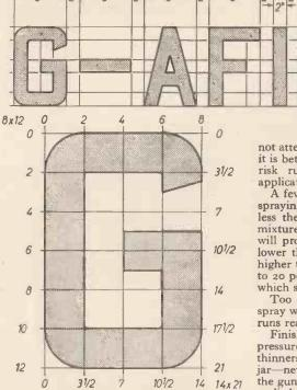
Fig. 79.-The thickness of the strokes in the letters is equal to the width of the spaces between the letters. The dash is made the full width of one letter as shown.
