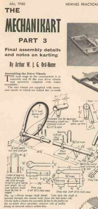
drive sprockets. The actual "drum" of the brake is a 7in. dia. "V" groove pulley. Two are required and they are obtainable from any large tool store or hardware factor. The pulley is bolted through the holes provided to the drive sprocket. Note that the flat side of the pulley (not the hollow face) should be against the sprocket.
