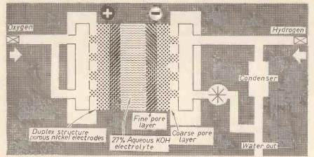
Fig. 6.—Cross section of a single cell.
