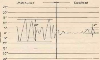
Fig. 10.—Reduction in rolling when using stabilisers.
