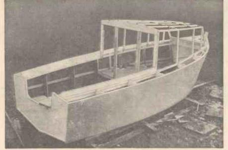
Fig. 24.—This stage shows the cabin framing and the cockpit coamings.
