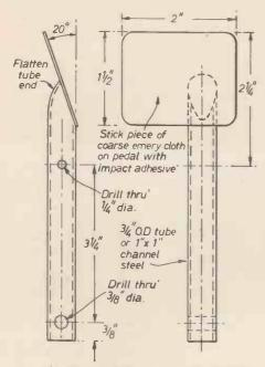
Fig. 25.--Detail of the foot pedals. Two are required, handed.
