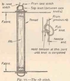
and wings, the stitches will all have their knots on the lower surfaces. Each knot must be tight and must not rely on the link to the next stitch for tension. If it is necessary to join the thread during stitching, arrange the join so that it can be pulled inside the surface to minimise irregularities on the external covering.
