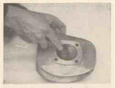
Fig. 9.-Removing carbon from the cylinder head with a screwdriver.
