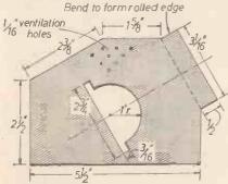
Make a left hand and a right hand side panel Fig. 3.-Layout of one of the sides.
