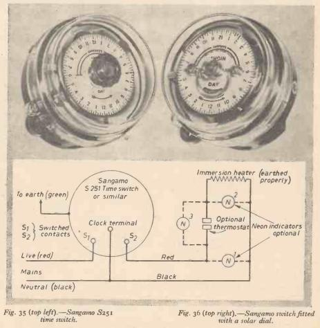
Fig. 37 (bottom).-Wiring to control an immersion heater.
