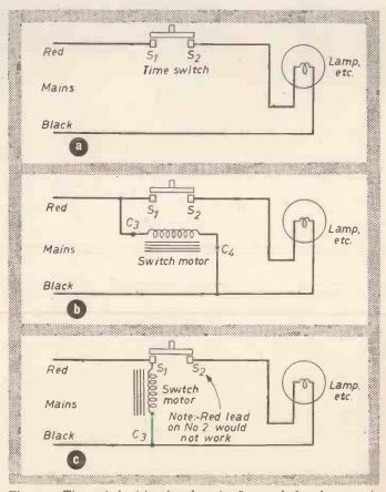
Fig. 42.—Time switch wiring (earth omitted); a—clockwork motor (2 terminals); b—synchronous motor (4 terminals); c—synchronous motor (3 terminals).
