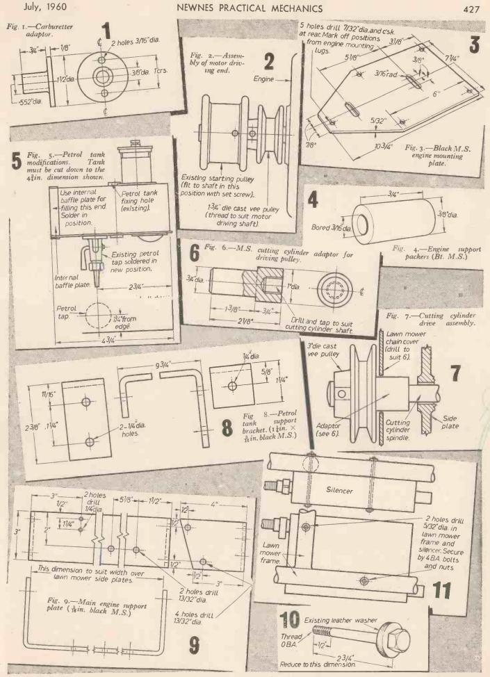
Fig. 10.—Modification to petrol tank fixing bolt.
