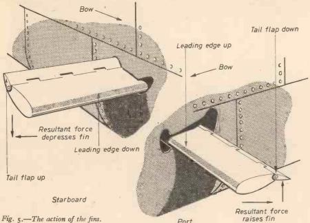
which, by hydraulic means, can be extended one on each side of the ship and tilted to create a turning moment to right the ship.
