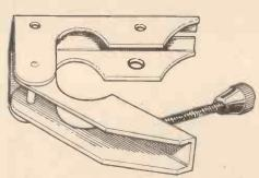
Fig. 3.—The type of clip most suitable for attachment to the draw tube.
