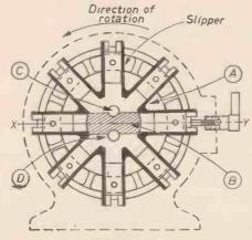
Fig. 4.—Variable delivery pump.
