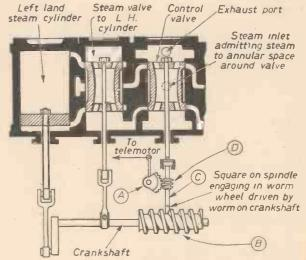
Fig. 3.-Valve gear of steam steering gear.
