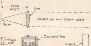
Fig. 1.—Finding the focal length of a lens.
