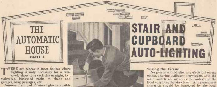
Automatic control of *indoor* lights is possible by foot pressure on floor pads at suitable places so that two-way throw-over type switches are operated at the start and finish of the journey. Provided two people do not cross, this is quite satisfactory and the apparatus is relatively simple.
