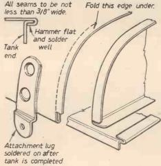
Fig. 59.—Details of the petrol tank construction.
