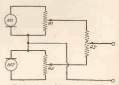
Fig. 6 .-- A more elaborate mixing circuit.
