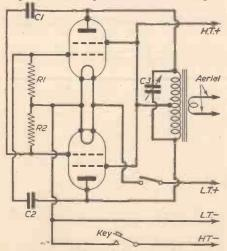
Fig. 1.—Two-valve battery operated transmitter.
