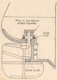
Fig. 1.—A balanced rudder.
