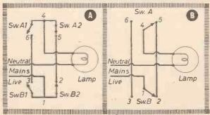
Fig. 3.—(A) Wiring of button switches for staircase lighting and (B) conventional two-way switching.
