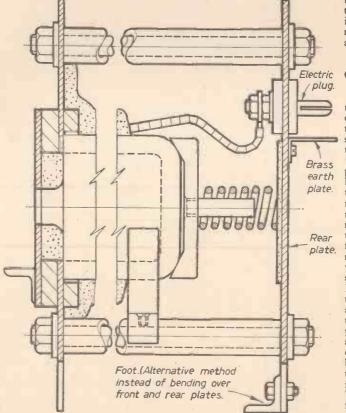
Fig. 2.—Sectional view of the front and rear ends of the furnace.
