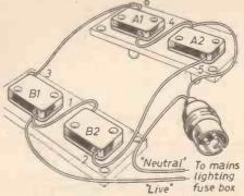
Fig. 2. - Wiring of button switches.
