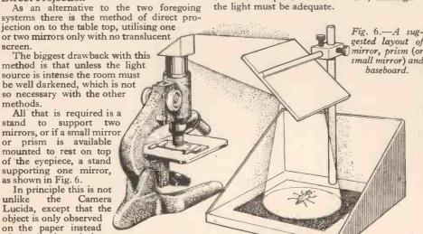
There is nothing very difficult about the construction of any of these projection systems for they can be made from sheet metal, wood or cardboard for a trivial sum of money, yet they will be of great value in drawing microscope objects.
