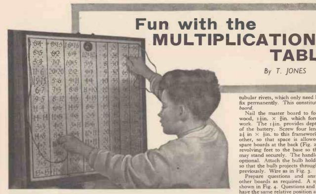
HE construction of the board is a simple matter and is based on the idea of a bulb being lit up when a correct answer is given. By using interchangeable boards, there is no limit to the variety of
