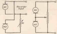
Figs. 4. and 5.—Two mixing Circuits.
