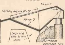
Fig. 5.—Side view of large projection unit for use with a strong light.
