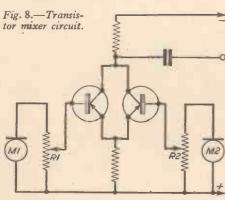
the variable resistance RI, which can control only one of the signals. In practice, the recorder input would be adjusted to receive the signal from MI, and then R, would be adjusted until M2 was balanced with MI. The value of RI depends, of course, on the impedances of the inputs.
