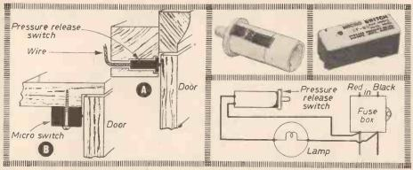
Fig. 4 (Left).—Cupboard switching; (A) using A55; (B) using micro switch. Fig. 5 (Top right).-A55 and micro switch. Fig. 6 (Bottom right).—Cupboard switch circuit wiring.
