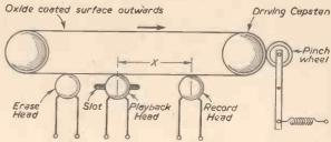
Fig. 10.—Magnetic drum replaced by endless loop of tape.
