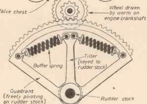
Fig. 2.—Steam steering gear.
