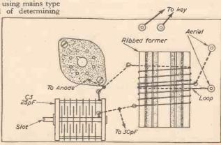
Fig. 4.—Mains transmitter layout.
