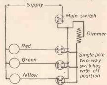
conjunction with a separate switch for each colour of lamp. If you require to be able to switch each lamp instantly from the dimmer to full strength, each outlet circuit could be controlled by means of a single-pole two-way switch as indicated above, each having an "off" position.
