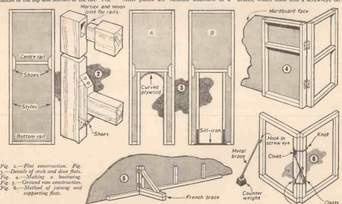
flat, and are forked at the other end to slot into a weight, may be purchased from any good theatrical supplier. There are also wooden extending braces, but quite serviceable ones can be improvised from a length of wood hinged at one end to the flat, and screwed into the stage at the other end.
