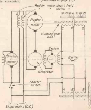
Fig. 7.—Electric steering gear.
