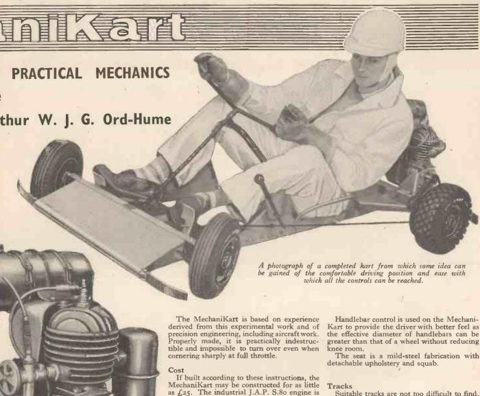
A view of the J.A.P. model JS8 two-stroke engine. Details of this engine are obtainable from the Villiers Engineering Co., Ltd., Marston Road, Wolverhampton. The silencer is discarded and an elbow exhaust pipe fitted.
