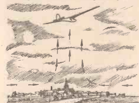
Fig. 3.—Glider flying in a thermal which has been started by the sun heating the air over a town.
