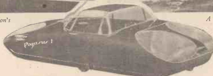
Pegasus I is a two-passenger, 850lb. car, designed for speedy travel 2ft. above land or water. It lands smoothly on small wheels.
