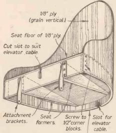
Three laminations of 1/8" short-grained ply glued to seat ply to support seat all round.
