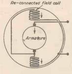
Fig. 7. — Reconnection of series field coils in parallel with each other.
