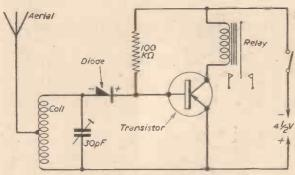
Fig. 2 .- The theoretical circuit.
