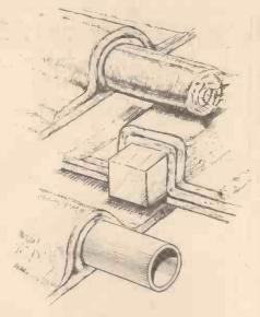
Fig. 5.—Three examples of bonded ribs for reinforcement.
