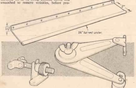
Fig. 14.—Window fittings. Shown here are a storm pelmet for opening-windows made from 20 s.w.g. aluminium, a window fastener and a friction stay-set: The spaces for the door and opening-windows should be primed and any holes stopped. They may then be undercoated to help seal the hardboard. One excellent finish for these edges is to glue strips of Formica along them.
