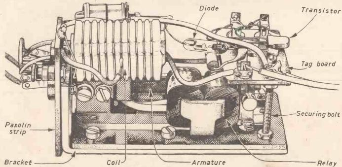
Fig. 1.—An enlarged perspective view of the completed receiver showing some of the principal wiring,
