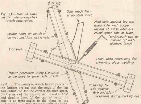
ing further are (a) that the ends of the leg and radius rod are the correct distance apart, (b) the axis of the leg and radius rod is true and dead in line, (c) the centre-line of the axle is at right-angles to the plane of the undercarriage so that the wheel will not "toein" or "toe-out," and (d) that the angle formed by the leg and the axis of the leg frame is ninety degrees.
