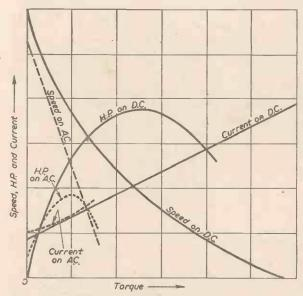
Fig. 5.-Operation of a particular series motor on D.C. and A.C.
