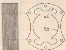
Fig. 4.—A laminated stator field system.
