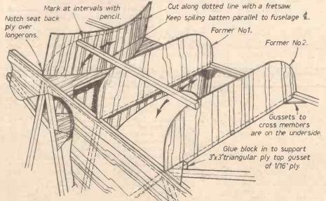
Fig. 42.—How to mark out the curve of the seat back former.
