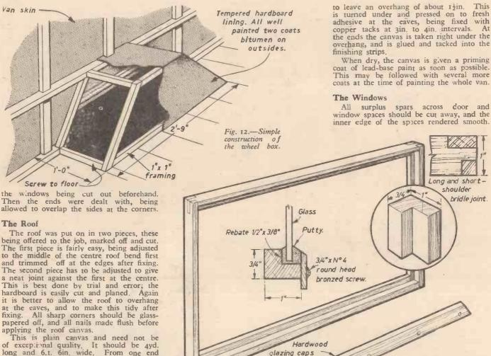
This is plain canvas and need not be of exceptional quality. It should be 4yd. long and 6.t. 6in, wide. From one end strips 4in, wide are cut, which are used first to seal the central joint, and any others if the roof has been put on in smaller
