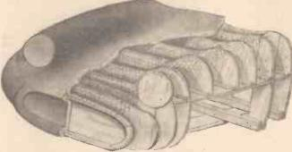
Fig. 4 (Left).—A typical temporary mould for moulding a car body.
