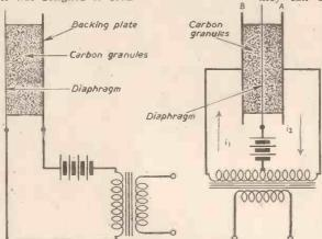
Fig. 1.—(a) Carbon microphone, (b) carbon microphones in push-pull.
