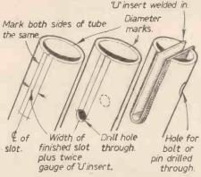
Fig. 37.—The three stages in marking out, cutting and finishing a tube fork-end.
