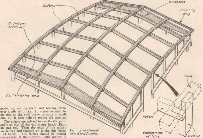
made, by wetting them and bracing them over a pile of bricks. It is not essential to do this as the roof curve is quite a small
