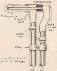
45 deg. wedge leaving about 4in, of metal to bend over when the join is soldered up airtight.
