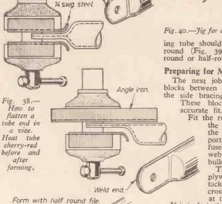
Fig. 39. — How meeting tubes are carefully filed to a
