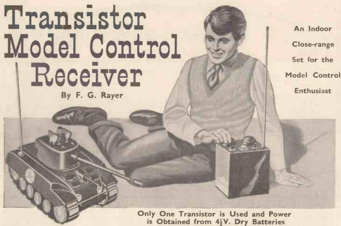
THIS receiver is for short range control only, and can be fitted in quite small boats or other models, as it is only approximately 1½in. × 1¾in. × 3in., including the relay. A good approximation of the size can be gained from Fig. 6. The current needed is under 2mA, at 4½V., and this can be obtained from three small dry cells in series.
