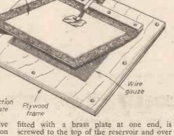
fitted with a brass plate at one end, is screwed to the top of the reservoir and over the delivery hole; a leather washer will make the faces airtight. The top surface of the feeder bellows where the foot is applied can be shod with an iron plate, a piece of thick rubber tread, or with strips of iron
