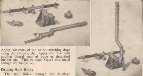
Fig. 41.—Control column and bracket assembly.
