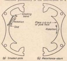
Fig. 10.—Modification of laminated field systems for operation on A.C.
