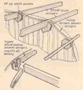
Fig. 43.—Attaching the stringers to the curved seat back former.
