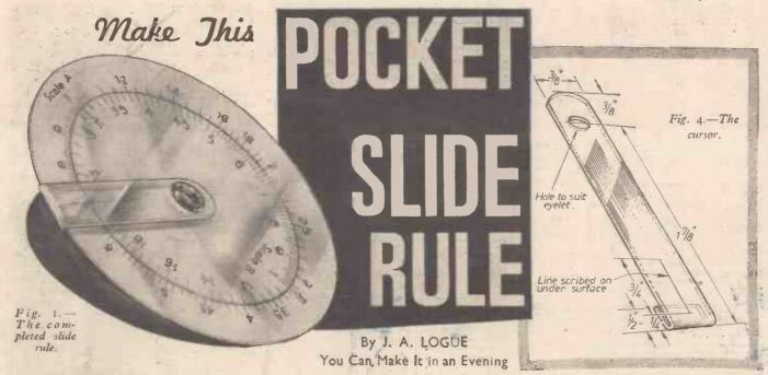
CIRCULAR pocket slide rule that can be used for making rapid calculations is shown in Fig. 1. Two scales are set out in black ink on thin tough white card. The graduations can be transferred from Figs. 2 and 3 on to tracing paper and then pricked through on to the cards. The lengths and numbering of the graduations are shown full size in the figures. Alternatively the scales as printed on this page can be used directly by pasting them on to thin card and cutting out along the lines shown.
