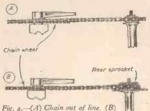
Chain correctly lined up on centre sprocket.
