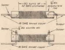
Fig. 3.-R.F. choke construction.
