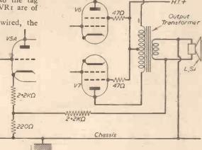
Fig. 21.—Modification to obtain 7 watts output.
