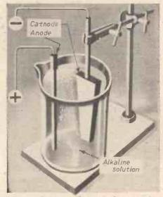
Fig. 6.—Apparatus for electrolytic cleaning.
