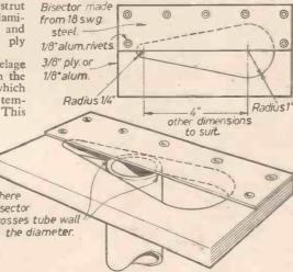
Fig. 36.—Tool for marking the diameter on a tube or circular bar.
