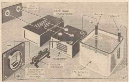
Fig. 1.—The electroplating circuit shown pictorially.
