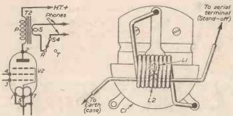
Fig. 4 (Left).—Alternative output circuit. Fig. 5 (Right).—Position of aerial.
