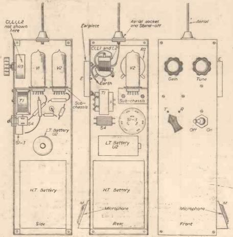
Fig. 8.-Internal and front panel layout.
