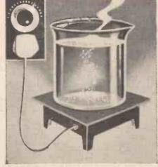
Fig. 4.—Apparatus for raising the temper of plating solutions.
