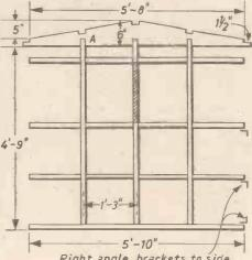
Right angle brackets to side Fig. 9b.—The end frame.
