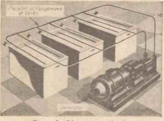
Fig. 2.—Parallel arrangement of tanks.
