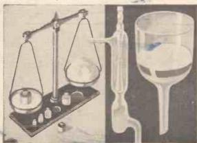
Fig. 5.—Balance, filter pump and Buchner fumiel.
