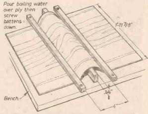
Fig. 32.—Pre-forming floor ply for seat cross support
