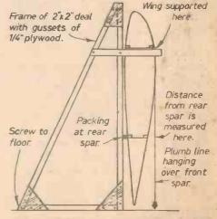
We' now come to the ply-covering of the alignment before ply-covering the leading edge.
