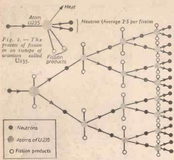
Fig. 3.—How neutrons cause more fission. This is known as a chain reaction.
