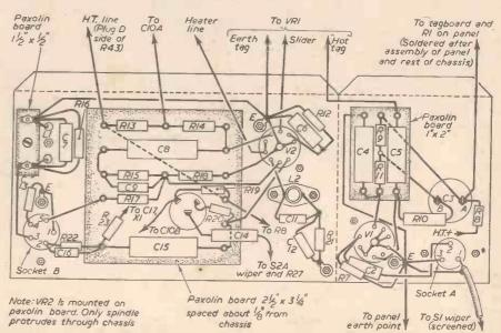
Fig. 19.—Wiring details of the pre-amplifier.
