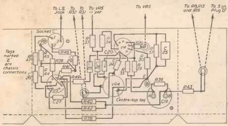
Fig. 17.—Mid-amplifier wiring.
