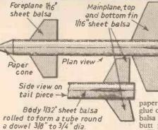
THIS model can fly over 60ft. The body is made by wrapping wood round an 8in. \*\* \( \frac{1}{4}\) in. dowel and butt jointing. Mark a sheet of 1/32in. balsa wood into four equal parts by means of three lines running along the length; these are to assist in aligning the fins. Soak it in warm water, wrap it round the former, bind in position and leave to dry. When dry cement the edges of the tube together.
