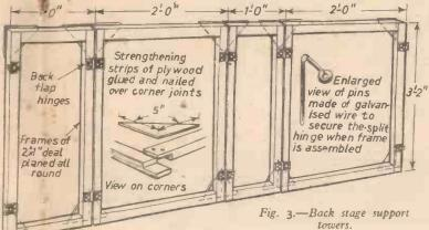
screwed together. Test the frames for squareness by measuring across diagonally. These dimensions should be equal. After the frames have been made square the triangular corner pieces are glued and nailed over the corner joints. For all constructional work on the stage it is advisable to use a waterproof glue such as Aerolite, so that if the stage is stored in the damp the joints will not be affected.
