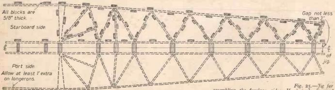
assembling the fuselage sides. If desired, diagonal bracing members may be located between headless nails. Longerons must be located in blocks.
