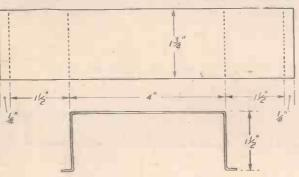
Fig. 7 .- Details and dimensions of the tagboard bracket.
