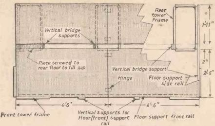
Fig. 10.—Dimensions for the floor of the stage.
