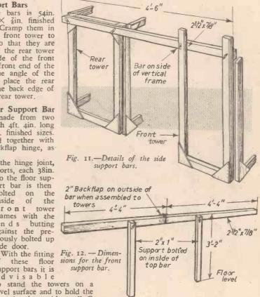
When the floors are placed in position on the stage there is a space left between the two so that the bridge supports, which are bolted to the sides of the rear support towers, may protrude above the stage level. This leaves a gap of about 2in, in between the floors which can be inconvenient to the operators when adjusting things in the wings. Because of this two pieces of deal 15in.  $\times$  2in.  $\times$  1in. are screwed to the front edge of the rear floor frames. This is shown in Fig. 10.
