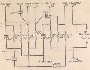
Fig. 6.—The tagboard connections.
