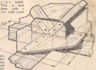
Remove the two sides from the assembly jig and plane off the surplus ply overlapping at the longerons. Do not as yet trim the excess from the unglued portion forward of the undercarriage member.
