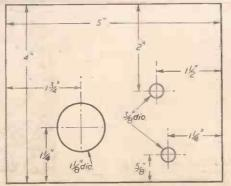
Fig. 9 .- Layout of the front panel.
