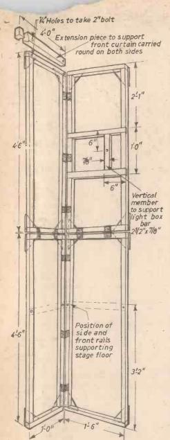
Fig. 8.—Details of left front tower.
