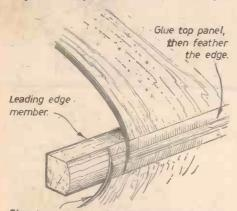
Glue bottom ply before feathering the edge. Fig. 24.—The joint between the top and bottom plywood panels covering the leading edge between ribs "C" and "D."
