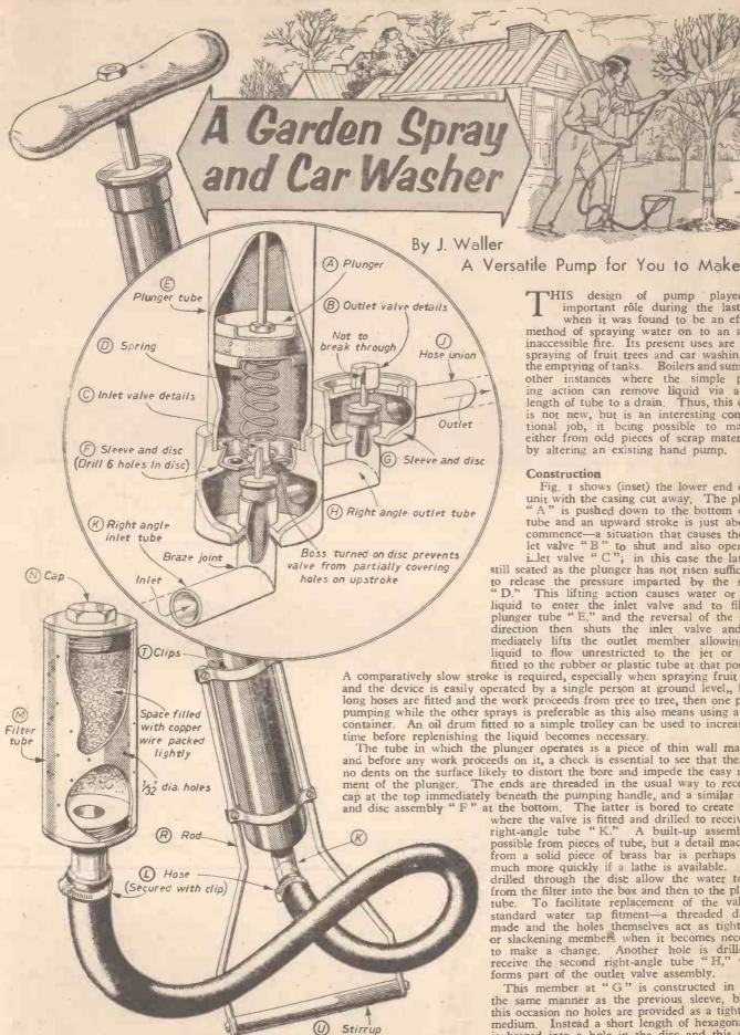
Fig. 1.—The completed pump with (inset) a cutaway view of the lower end. Part of the filter casing has also been removed.
