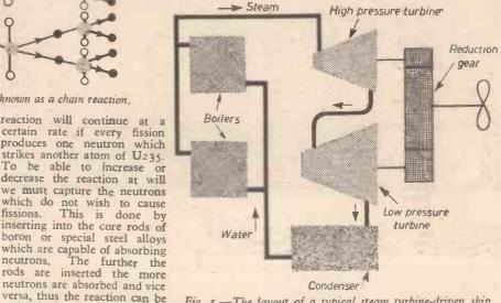
Fig. 5.—The layout of a typical steam turbine-driven ship.
