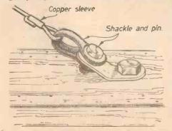
Fig. 21.—Attachment of bracing wires. The other end of the wire is fixed with a turn-buckle.
