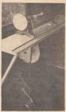
Fig. 2.—The completed pedal powered lathe.
