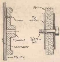
Fig. 3.—Details of the flywheel sander and radial buff.
