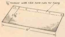
Fig. 14.—Main dimensions of the metal panel. given therefore in the panel sketch of Fig. 14, apart from those of overall size and fixing points.
