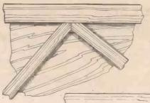
Fig. 26.—(Left) typical between bracing and longeron in fuselage sides and (below) joint of heavy undercarriage member and cockpit bracing struts in fuselage sides.
