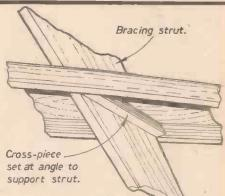
Fig. 3.—Method of attaching the bracing struts where they pass through a rib.
