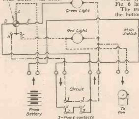
Fig. 13.-Wiring diagram of the simplified open circuit alarm.
