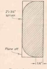
Fig. 6.—Section through tailplane front spar
