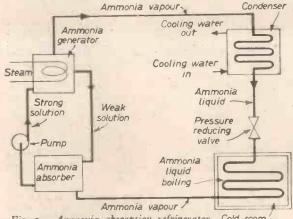
Fig. 3 .- Ammonia absorption refrigerator. Cold room
