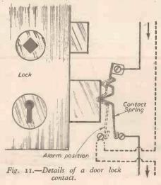
sight, can be employed. The contact spring is kept pressed down on to point 2 as long as the window is closed, but when opened the contact spring touches point 3 and the alarm is given.
