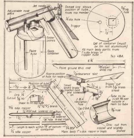
Fig. 1.—A cut away perspective view and details of the spray gun.
