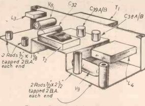
Fig. 6.—Positions of the rod spacers.
