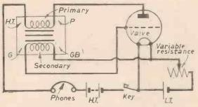
Fig. 4.—The theoretical circuit.
