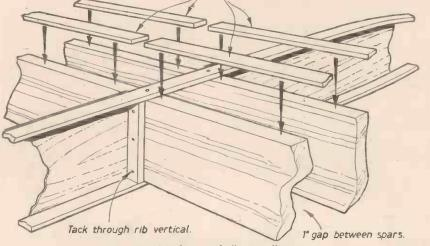
Fig. 9.-Attachment of ribs to tail spars.
