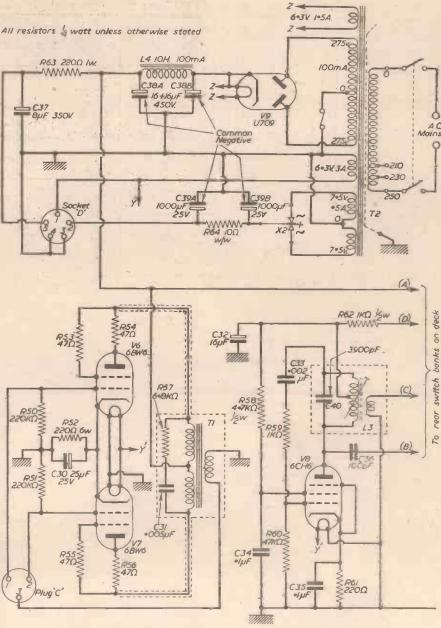
Fig. 2.-Circuit of the output stage, bias oscillator and power unit.
