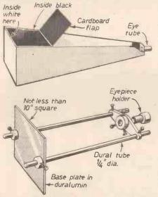
Fig. 2.-Simple sun projection box made from card.
