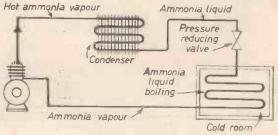
Fig: 4:-Vapour compression refrigerator.
