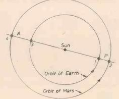
Fig. 8.—Orbit of Mars. P-Perihelion. A-Aphelion. When Earth and Mars are at positions 1 and 2 the opposition distance is about 35 million miles and at positions 3 and 4 it is 62 million miles.
