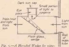
Fig. 5.—A Herschel Wedge for view-ing the Sun at the Newtonian focus.
