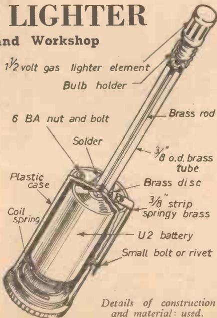
Details of construction and material used.
