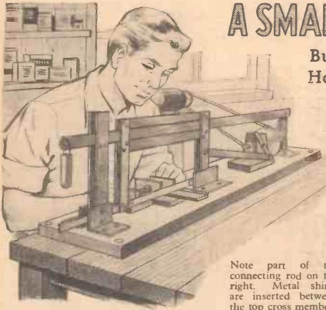
**T**HIS machine, of which Fig. 1 gives two views, is referred to as a small power hacksaw for the reason that it employs a 9in. blade instead of the more normal 14in. In all other respects, it is a sturdy and powerful machine capable of dealing with work up to 4in. wide and of any reasonable depth.
