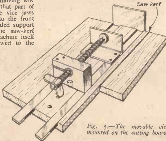
Fig. 5.—The movable vice mounted on the cutting board.
