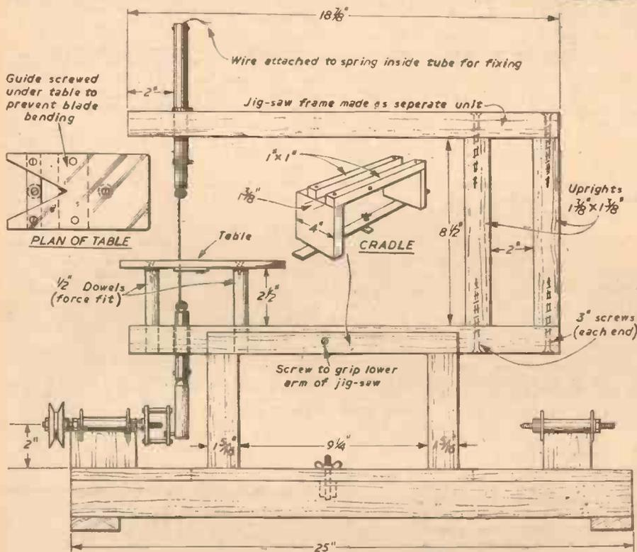
Fig. 1.—General arrangement of the jig-saw and details of the modified lathe.
