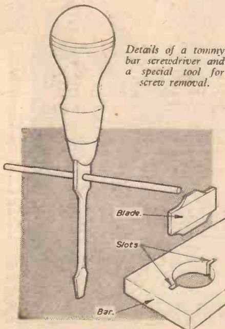
Details of a tommy bar screwdriver and a special tool for screw removal.
