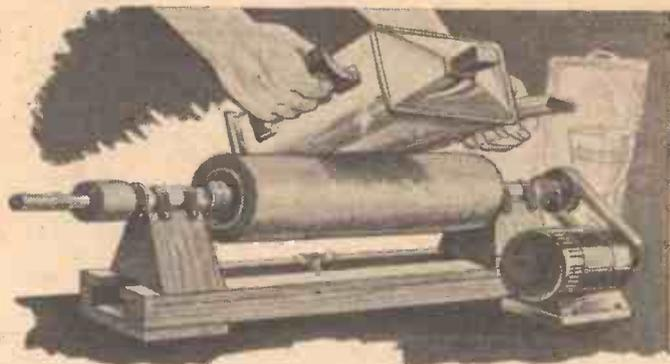
Fig. 4.—The buffing machine set up for polishing household cutlery, etc.
