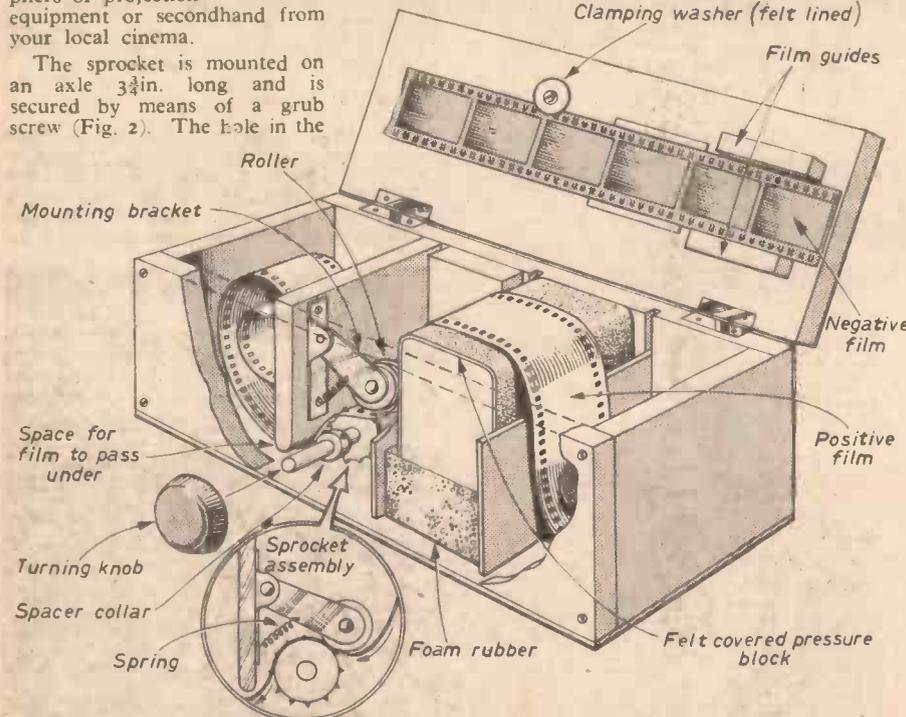
Fig. 2.—General arrangement of the printer, showing method of threading film through.
