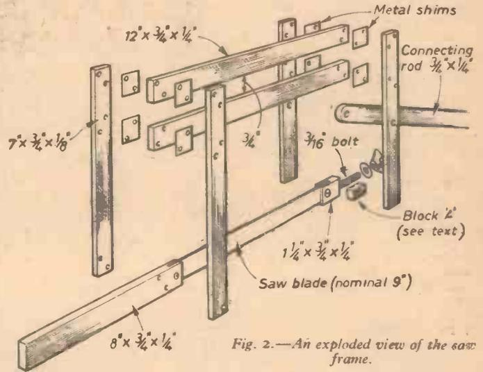
Fig. 2.—An exploded view of the saw frame.
