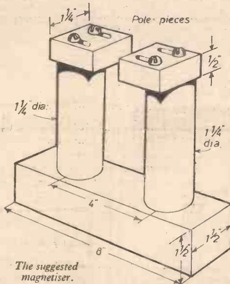
screwed together. The pole pieces could be secured by means of screws through slots, if required, so that the distance between the pole pieces can be made slightly less than the length of the rods to be magnetised. Each pole could be wound with about 3 1/2 lb. of 16 s.w.g. D.C.C. copper wire, the two coils being connected in parallel with each other for use from a 6-volt car accumulator. Care must
