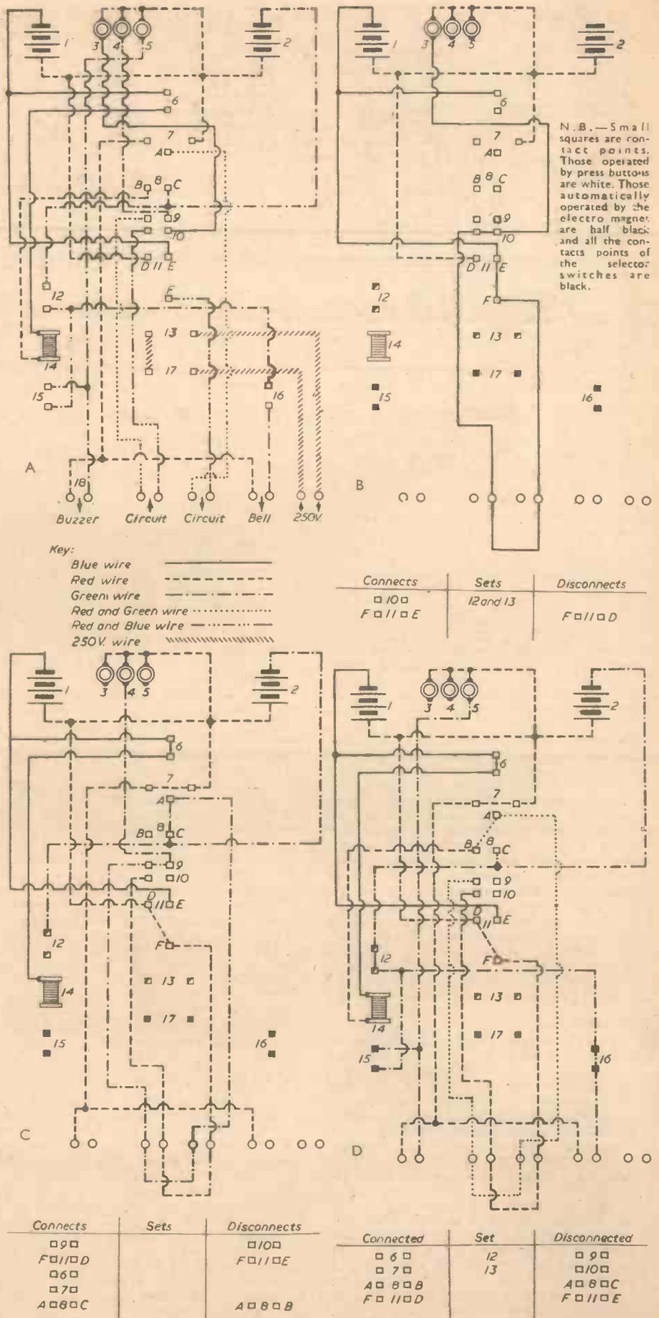
Fig. 7.—(A) complete wiring diagram; (B) black button pressed down; (C) red button pressed down; (D) unit switched on and alarm at set position.
