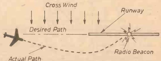
Fig. 4.—How an aeroplane may land at an angle to the runway if the pilot "homes" on a radio beacon when a cross wind is blowing.
