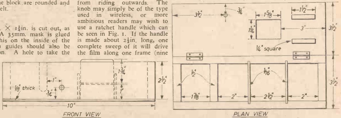
Fig. 3.—Front and plan views of the box giving dimensions.
