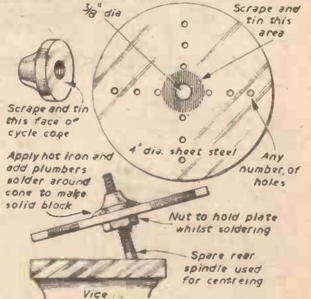
Fig. 7.—The method for soldering the cycle cone to the faceplate.
