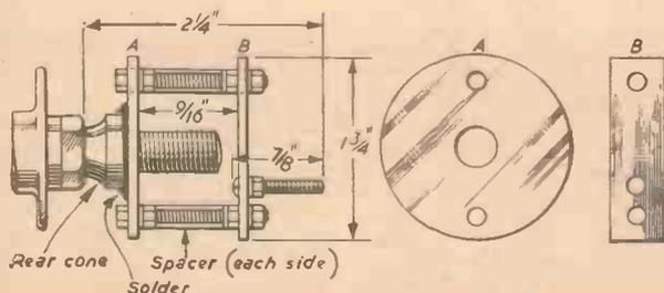
Fig. 2.—Details of the eccentric device.
