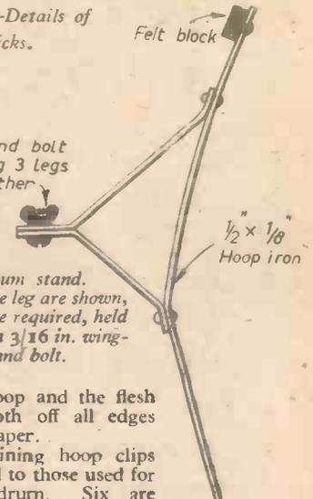
Fig. 9.—Drum stand. Details of one leg are shown, but three are required, held together by a 3/16 in. wing-nut and bolt.
