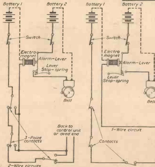
Fig. 2.—The theoretical "open" (left) and "closed" circuits.
