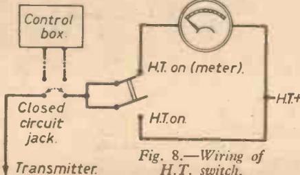
from which it may be seen that when the meter is out the toggle serves as an on-off or keying switch.
