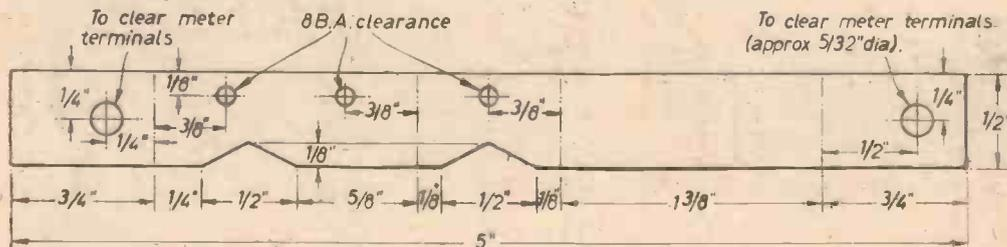
Fig. 1.—Dimensions of the frames.
