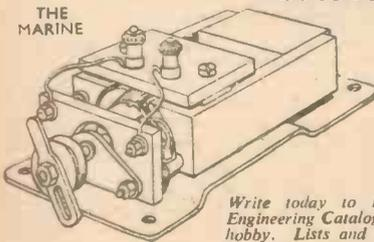
The Marine motor is a powerful permanent magnet unit suitable for model boats up to 39 ins. long and will give many years' service. It will operate from two 3-cell dry batteries coupled in series or from a 6-volt accumulator. Length 3 1/2 ins. Width 2 ins. Height 1 1/2 ins. Weight 11 1/2 ozs. Price 63/-.
