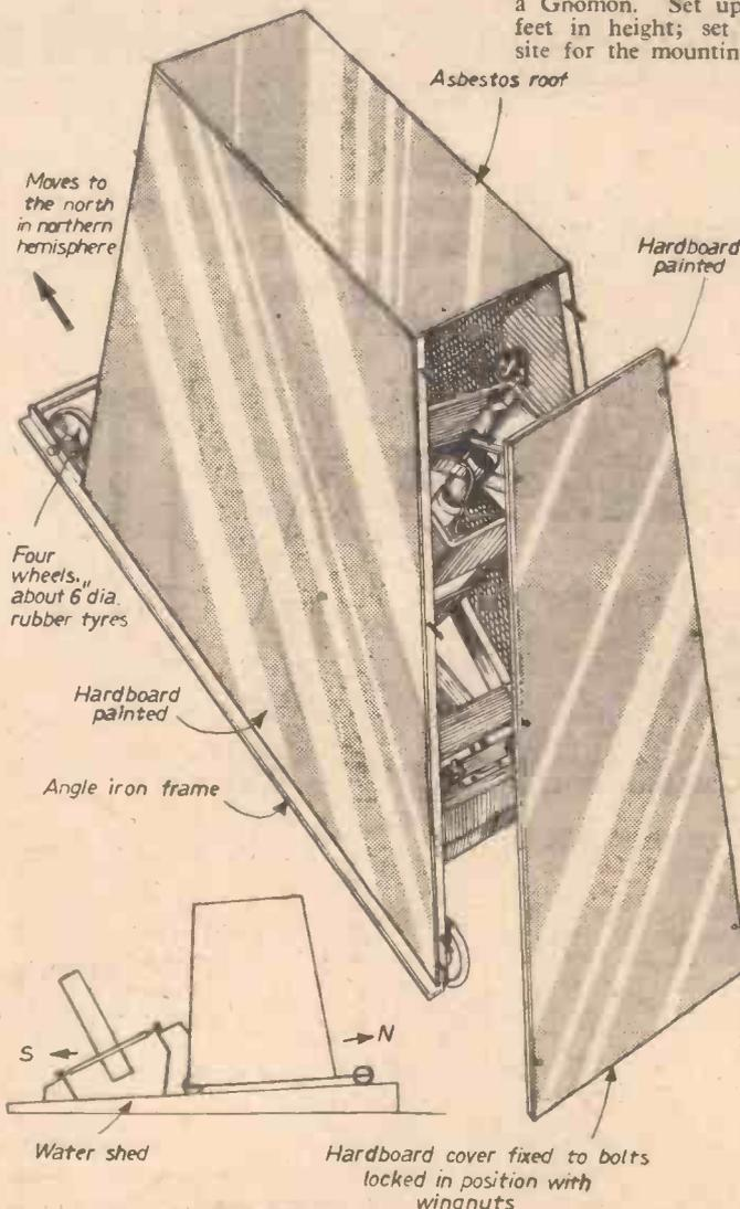
Fig. 1.—A simple run-off shed to protect the cradle-mounted telescope.
