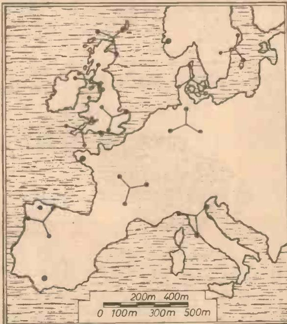
Fig. 2.—Map showing position of Decca Navigator transmitters (tripod symbols) and Consol stations (shown as blobs).
