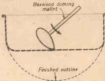
Fig. 2 (Right).—First stage in hollowing the bowl.
