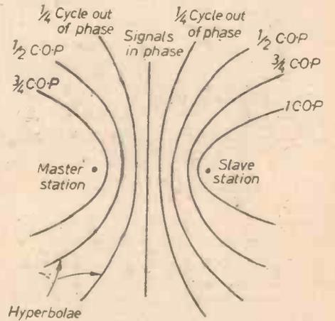
Fig. 9.—Two stations transmitting on the same frequency form lines where the degrees of out-of-phase is the same.
