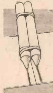
Enclosing the joint with wax crayon lines.
