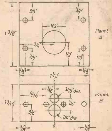
Fig. 4.—Details of the Paxolin panels; all holes are 8 B.A. clearance except where marked.
