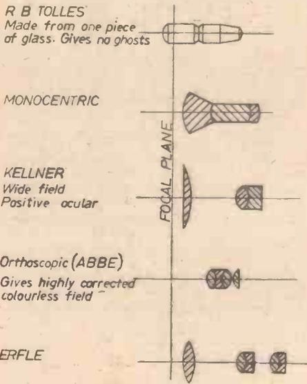
Fig. 5.—Details of the optical train and suitable eyepieces.
