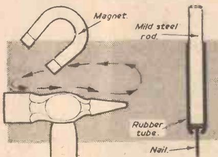
ONE way of accomplishing this feat is to use a magnetic hammer. Any hammer can be magnetised, using an ordinary permanent magnet and dragging it along the hammer-head as shown in the sketch above. A simple tool for this job is shown above right. It can be easily made by anyone from an old piece of rubber tube and a
