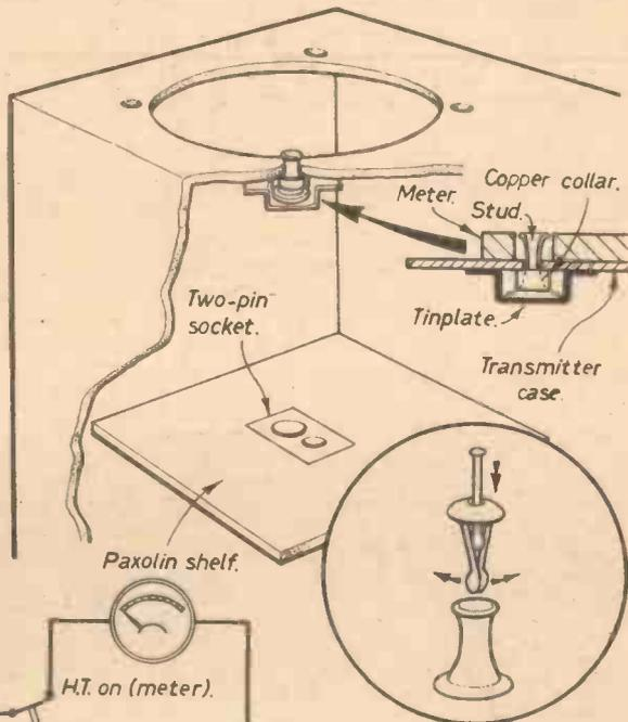
Fig. 8.—Wiring of H.T. switch.
