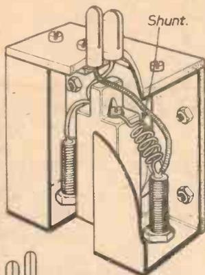
Fig. 7 (Right). — Method of fixing meter, with (inset) action of stud.
