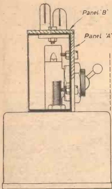
Fig. 5 (Above). — Side view showing adjustment of switch. Wiring is omitted for clarity.
