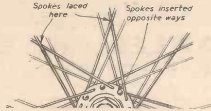
Fig. 2.—How spokes are laced
