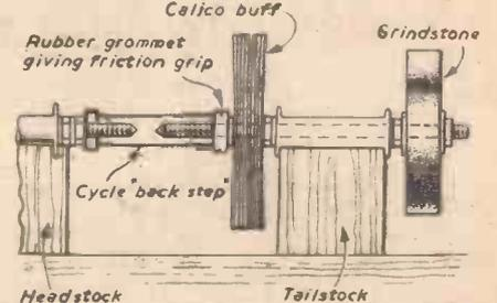
Fig. 8.—Calico buff and grindstone mounted on the lathe.
