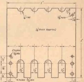
Fig. 5.—Dimensions of asbestos board resistor support.
