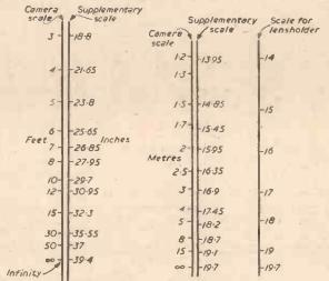
Fig. 1. Feet scale with 1 dioptre lens.
