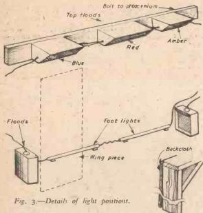
three colour system. As all illumination will be done by electricity, it is obvious that the work of equipping the theatre with wires and light points should be done, from start to finish, by an expert on the subject, in order to ensure a system both shock-proof and
