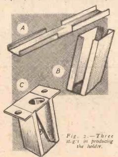
as the block and about in. wider. The metal and block are clamped together in the vice, the metal overhanging the block by an equal amount on each side. The metal is then formed over the block to give the chan-nel section shown at "A" in Fig. 2. The centre section is then cut away. The size of this section will depend on the size of the particular sharpener being used by the reader.
