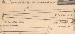
Fig. 1.—Taper jig details.
