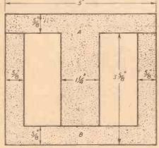
Fig. 2. Dimensions of transformer gore stambines.
