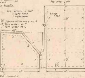
Fig. 9 .- Marking out and cutting the hood fabric.
