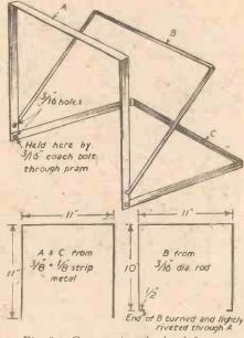
Fig. 8.—Constructing the hood frames.
