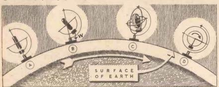
Fig. 6.—The gyroscope is made north seeking.
