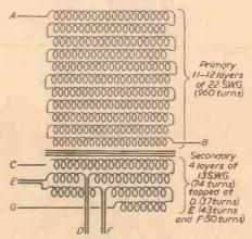
Fig. 4.—Details of transformer winding.
