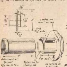
Fig. 17.—Eyepiece draw tube assembly.
