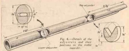
windway opening, is centred 3 3/16in. from the base of the instrument. Drill windway it 3/16in, dia, and open out gradually to produce the note E.
