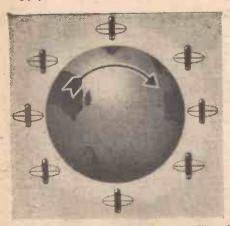
Fig. 4.—Gyroscope at the equator directed east and west and the earth rotating.
