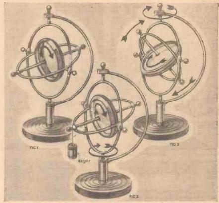
Fig. 1.—The gyroscope. Fig. 2.—A weight attached. Fig. 3.—The gyroscope turning bodily in a vertical plane.
