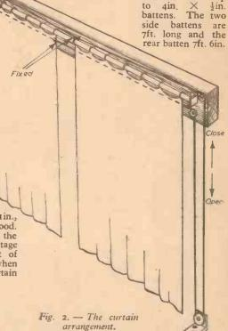
The two drapery supports are each 7ft. 1½in. × 1½in. and are joined at the centre by a flat metal strip bolted to each. An alternative system would be to fit a square
