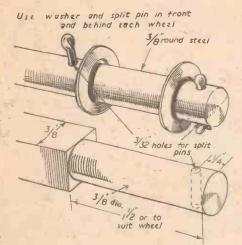
Fig. 4.—Two methods of fixing the wheels.
