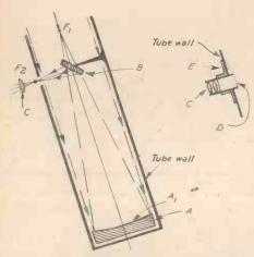
Fig. 1.- The optical system of the Newtonian reflecting telescope.
