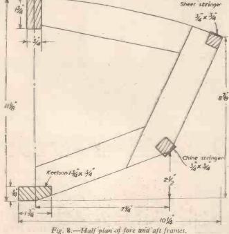
Side member of cockpit Sheer stringer Top part of fram sawn out to fit side member of cockpit Pieces on both sides of frame to secure joint Chine stringer 81/2 Keelson -13/4 10 76 1376
