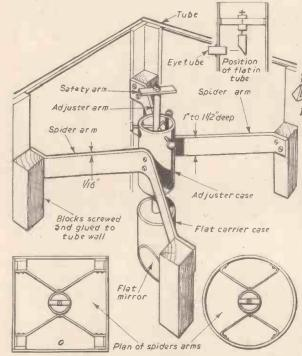
Fig. 7.-Holding and adjusting the optical flat holder.
