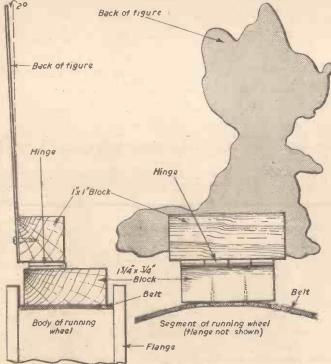
Fig. 7.-Fitting the figures on to the belt.
