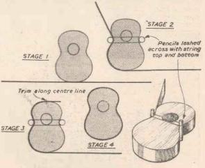
Fig. 2.-Four stages in fitting the sides.
