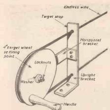
Fig. 10.- The target mechanism at firing point.
