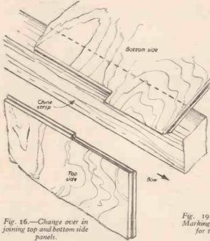
jointing compound is used under the keel so that any gap in the joint between the panels will be filled.
