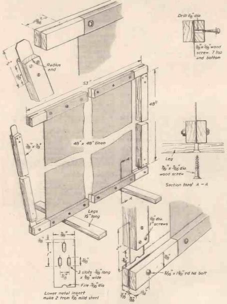
Fig. 1.-Full details and dimensions for construction.
