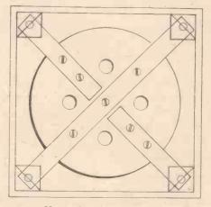
Fig. 4.—Underside of mirror cell in a square tube.
