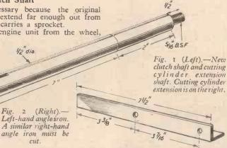
take off the cover and the flywheel. If the flywheel is off any length of time, remember to load it up with iron (hammer head, nuts, spanners, etc.) to keep in the magnetism. Remove the screws holding the two halves of the chain casing and open it up. This exposes the clutch unit and its driving chain. By undoing the 5/16 in. nut in the centre of the clutch, and careful use of a hammer and drift, the clutch shaft can
