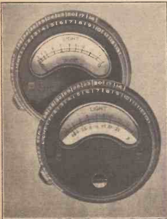
An unmodified meter (above) and meter with new scale added.
