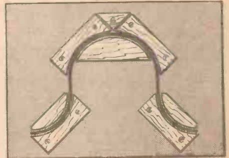
Fig. 5.—A plastic and plywood "sandwich."
