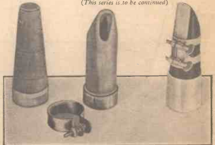
Fig. 11.—On the left are shown two stages in making the mouthpiece, right is a commercial mouthpiece. A reed clip is shown in the foreground.
