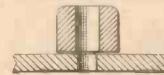
Fig. 8 (Above).—Showing an undersized hole in the Perspex and clearance hole in the attachment.
