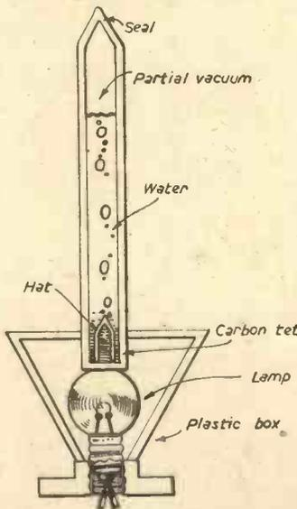
Fig. 2.—A completed bubble tube.
