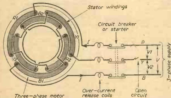
Fig. 1.—Connections of a three-phase motor with open-circuit in one phase.
