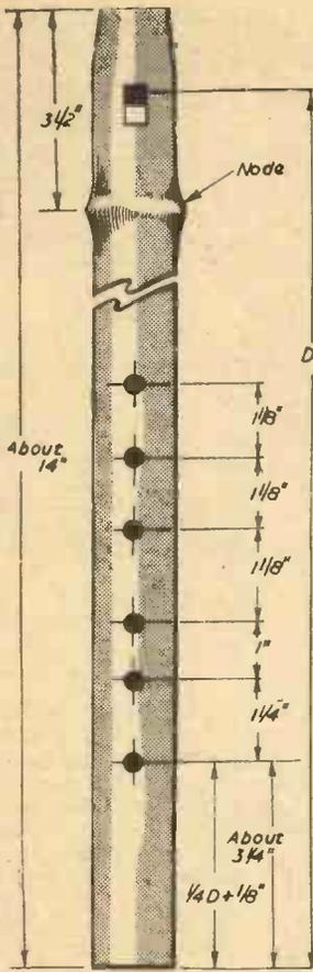
Fig. 31.—Finger holes for the alto pipe.
