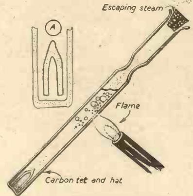
Fig. 3.—The filling operation.
