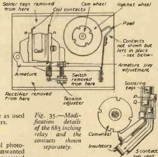
Fig. 35.—Modification details of the 685 inching relay and the contacts shown separately.
