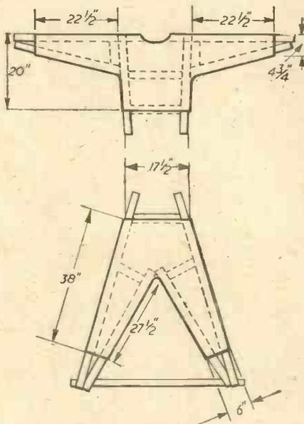
Fig. 7.—How the garments are stretched over the frames.
