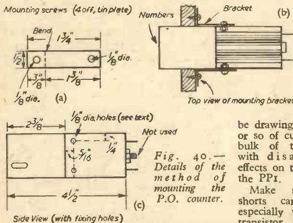
Fig. 40.—Details of the method of mounting the P.O. counter.
