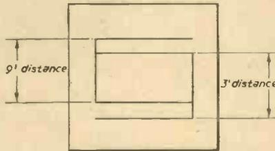
Fig. 2.—Details of reflex screen.
