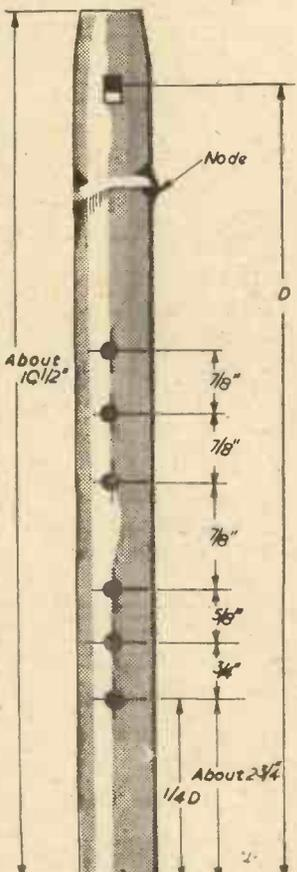
Fig. 28.—Finger holes for the treble pipe.
