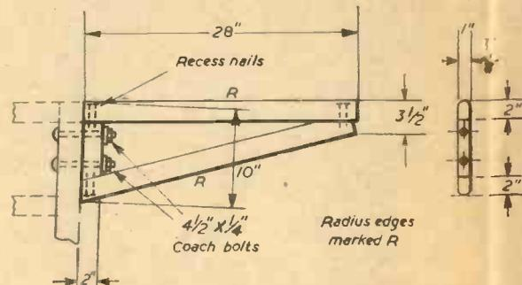
Fig. 3.—Details of the arm-piece.
