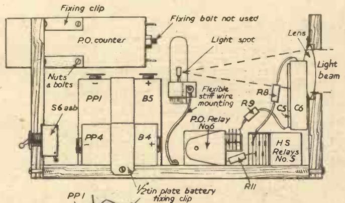
Fig. 41.—Side view of photo counter, showing the layout of components.
