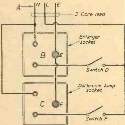
Fig. 2.—Distribution panel wiring.
