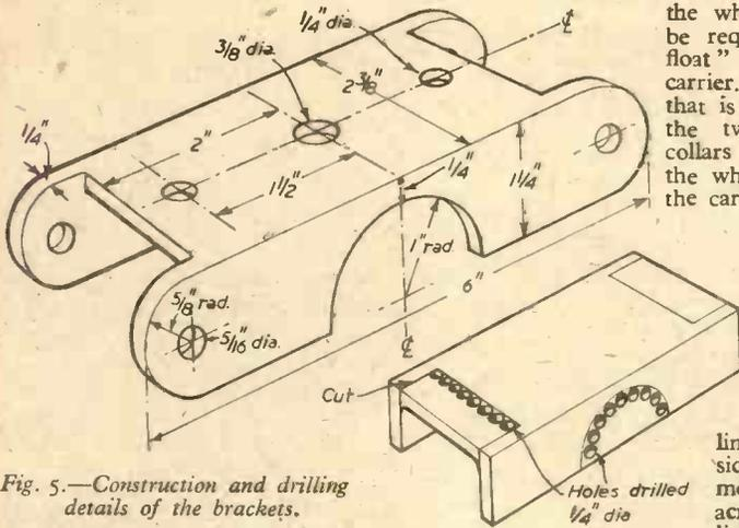
Fig. 5.—Construction and drilling details of the brackets.
