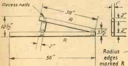
Fig. 4.—Details of the leg-piece.
