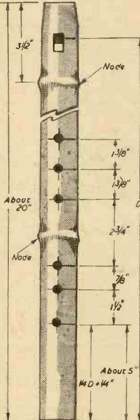
Fig. 33.—Finger holes for the tenor pipe.
