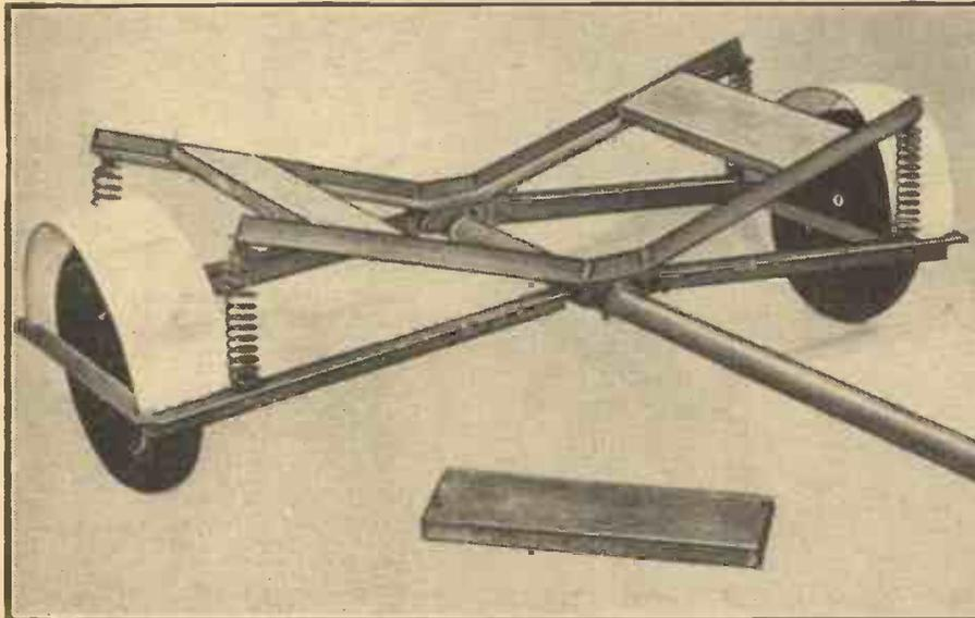
Fig. 11.—(Above) The finished trailer showing mudguard details.
