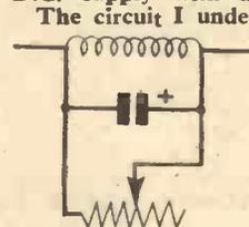
I have experimented with a 6,000 ohm relay 250. μF 25 v. wkg. condenser and 25 k wirewound resistor. Can these values be reduced or improved for more accurate and positive action? I understand condensers are either not accurate or tend to lose their accuracy. Could you estimate the number of operations likely before this becomes serious?—R. Harrison (Southport).
