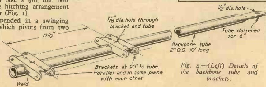
Fig. 4.—(Left) Details of the backbone tube and brackets.
