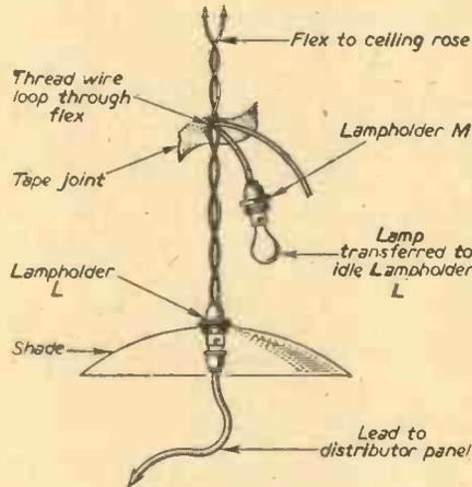
Fig. 4.—Using an "idle" lampholder.
