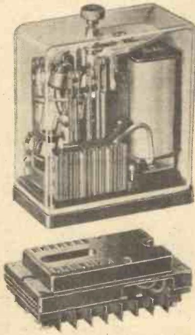
The new C.F. and S. Plug-in relay.
