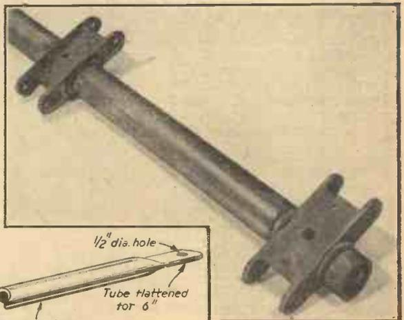
Fig. 3.—(Above) The completed brackets welded to the backbone tube
