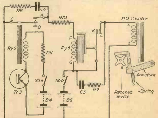
Fig. 37.—Circuit of the electronic transistor counter.
