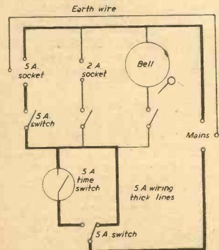
Fig. 3.—A modified circuit for a three-pin plug.
