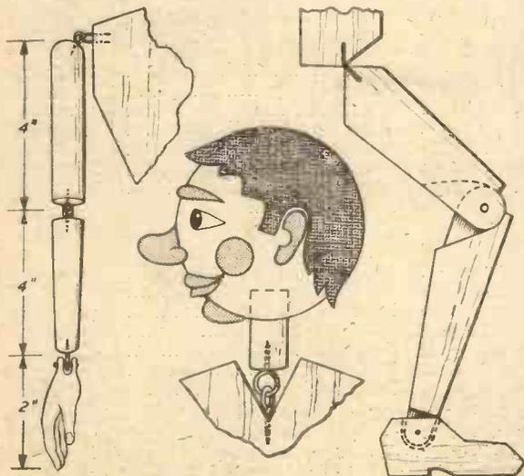
Fig. 3.—Details of the knee, ankle, arm and head joints.
