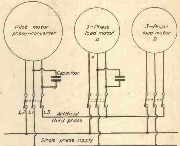
Fig. 4.—Use of phase-converter for feeding three-phase motors from single-phase mains.
