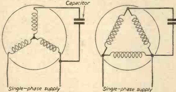
Fig. 3.—Capacitor methods of starting three-phase motors on a single-phase supply.
