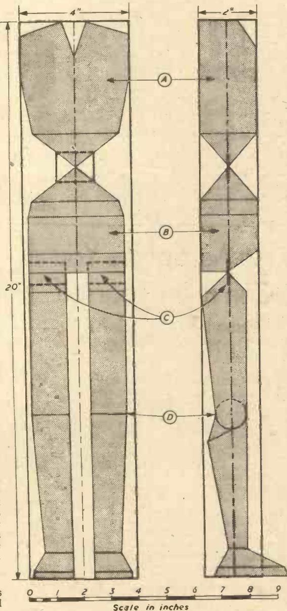
Fig. 2.—Details of the body and legs.
