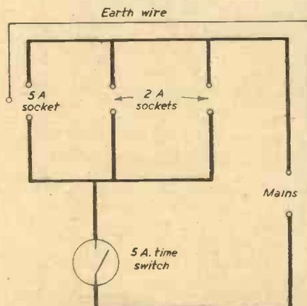
Fig. 4.—A simple circuit for when the alarm is not included in the box.
