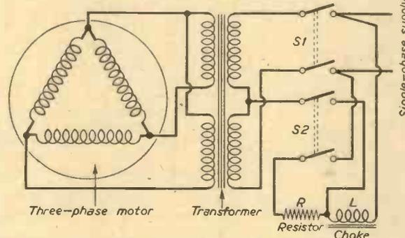
Fig. 2.—One method of starting a three-phase motor from a single-phase supply.
