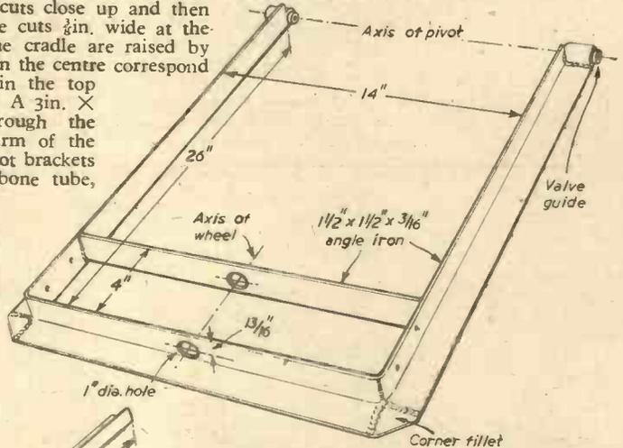
Fig. 6.—Angle iron to the above dimensions is employed to make the swinging arm frames.
