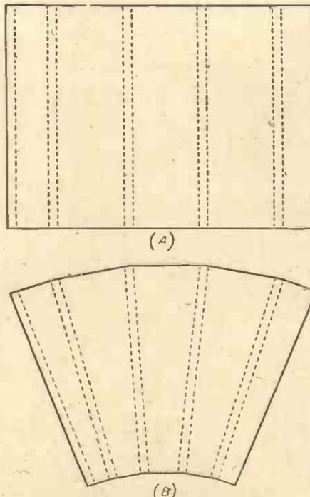
Fig. 2.—Marking out the bellows.
