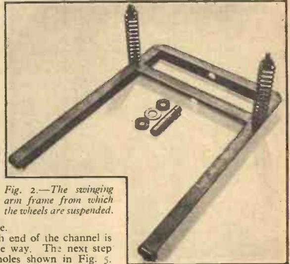
Fig. 2.—The swinging arm frame from which the wheels are suspended.
