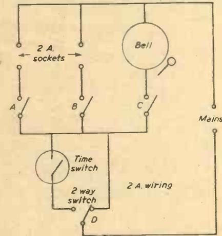
Fig. 2.—A suitable circuit for a prototype time switch.
