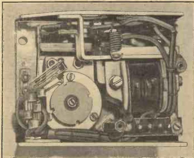
Fig. 36.—A top view of the unmodified 685 inching relay.
