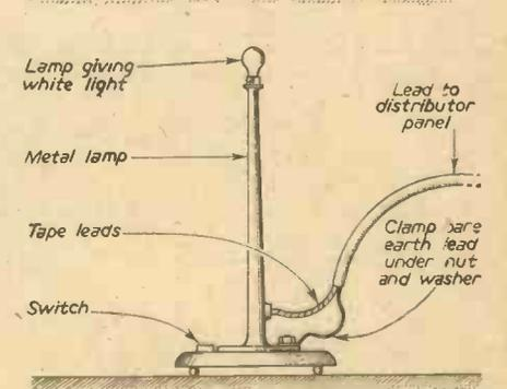
Fig. 5.—Electrical precautions in the improvised darkroom.
