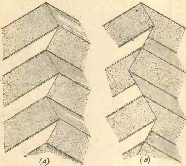
Fig. 1 (A).—Type of bellows most commonly seen; (B) An older type still in use on some cameras, etc.
