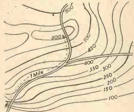
Fig. 1.—Measuring a gradient.
