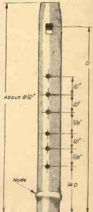
Fig. 35.—Finger holes for the soprano pipe.
