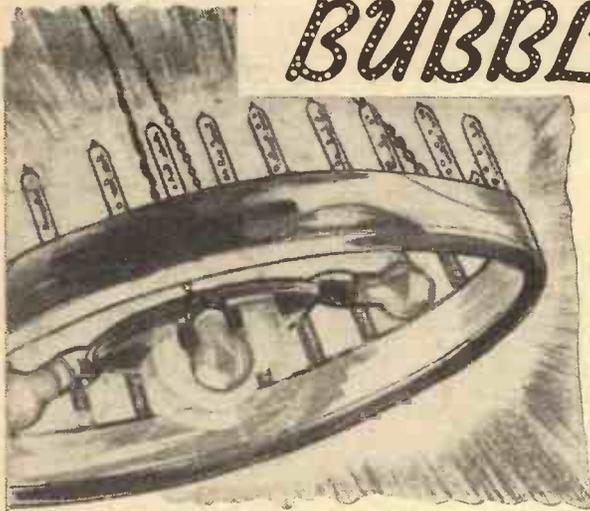
**M**OST people must have seen these lamps at some time and watched the endless trail of bubbles passing up through a coloured fluid. It is not generally realised, however, that they may be easily made at home with little more than a length of glass tube and a suitable gas jet. Moreover, once the working principle has been grasped, they are capable of many novel designs.
