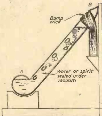
Fig. 1.—The simplest form of bubble tube.
