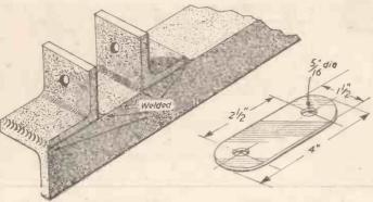
Fig. 6 .- Bearing for the front end of the spring.
