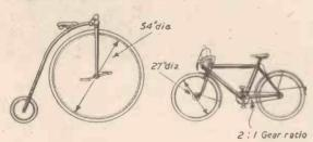
Fig. 1.—How the present system of expressing cycle gears originated.
