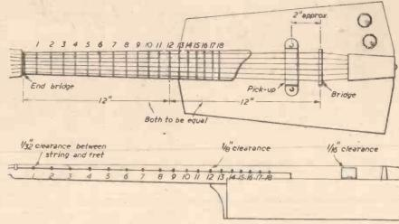
Fig. 7.—Position of bridge and clearances for strings.
