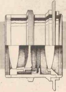
The Zeiss Novar triplet.
