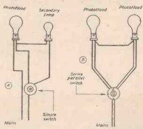
Fig. 2 .- (A) Using a secondary lamp and (B) wiring in parallel.
