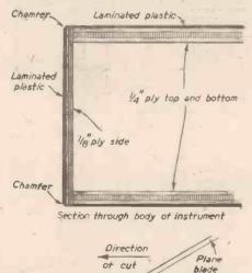
Fig. 4.—Section through the body showing how the plastic is glued and chamfered; also the arrangement of the plane blade for cutting.
