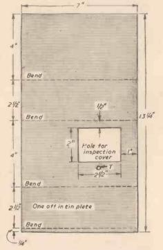
Fig, 10.—Cutting and bending plan for the tinplate cover.
