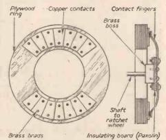
Fig. 26.—Method of making contacts.
