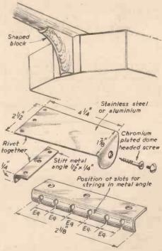
Fig. 2.—Details of the shaped block, tail-piece and metal angle.
