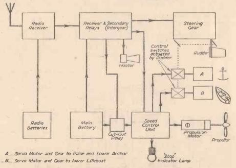
Fig. 30.—Block diagram of system.
