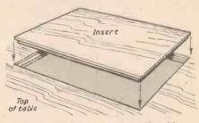
Fig. 6.—Renewing cutter-gap in table.
