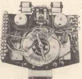
Fig. 28.—Rear view of speed control switch showing contact assembly, reversing relay, suppressing condensers and tag strips for connecting inputs and outputs.
