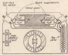
Fig. 25 .- Contact side of speed control switch.
