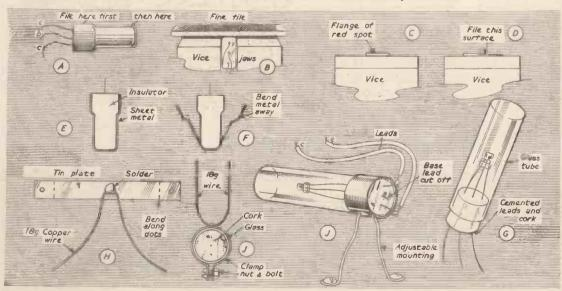
Fig. 2.—Modifying a red-spot transistor.
