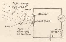
Fig. 1.—Germanium diode as a photo-cell.
