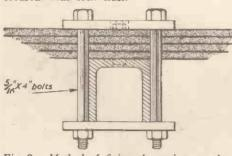
Fig. 8.—Method of fixing the springs to the axle bar.
