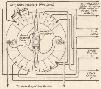
Fig. 27.—Suggested wiring of speed control unit. A—Full-speed ahead; B—Half ahead; C—Slow ahead; D—Stop (mast lamp on); E—Half speed astern; F—Effect channel 1; G—Ditto 2.
