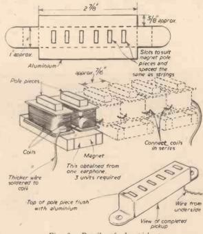
Fig. 8.—Details of the pick-up.
