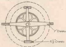
Fig. 2.-With 7in. cranks the feet travel in a larger circle than with 61in. cranks and therefore travel further for the same amount of forward distance travelled.
