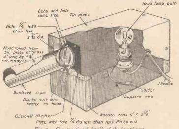
Fig. 9 .- Constructional details of the lamphouse.
