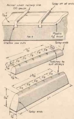
Fig. 6.—Details of frets and bridges.
