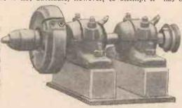
Fig. 2.—The working parts of the spindle moulder.
