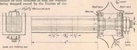
Fig. 4 (Left),—The axle is shaped to fit inside the channel. Fig. 5 (Right).—Fitting the wheels.
