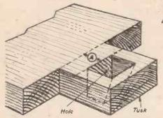
Points to remember are that the tusk must be long enough to pass through the side member and provide ample timber in which the hole can be cut, and, once the hole has been cut, that there is enough timber around it to withstand the driving of the wedge. Another point, and a very
