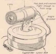
Fig. 29.—Details of the lamp.
