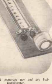
Fig. 22.—A prototype wet and dry bulb thermometer.
