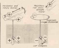
Fig. 12.—Giving a positive charge and checking it.
