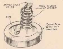
Fig. 28.—Bimetal assembly for the heat ray detector.
