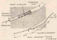
Fig. 2.—(a) Coaxial type cable. (b) Preparation of coaxial cable.
