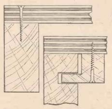
Fig. 6.—Two methods of fastening the top to the rails.
