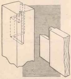
Fig. 1 .- Jointing the rails into the corner legs.
