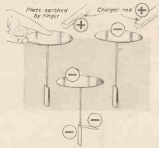
Fig. 10.—How to give a negative charge.
