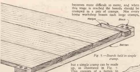
the boards are placed so that this grain funs in opposite directions in each pair of boards. When glued up as shown the finished job will be very much less liable to warp.
