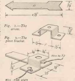
Fig. 4.—The lampholder connections
