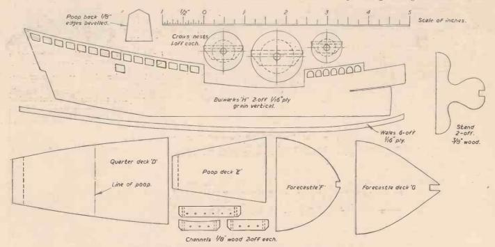
Fig. 8.—Constructional details of the bulwarks, superstructures, etc.
