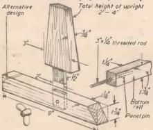
Fig. 2.—Details of the lower ends.
