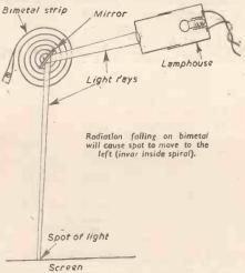
Fig. 33.—Plan of detector ready for use.
