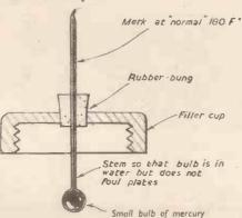
Fig. 24.-Motor vehicle thermometer.
