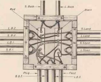
Fig. 3.—Internal wiring of junction box. Black wires are shown black and red wires shaded.
