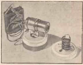
Fig. 30.—Heat ray detector complete (less screen).
