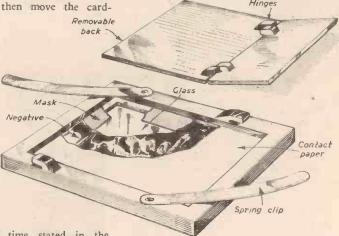
Fig. 2.—A typical contact printing frame.
