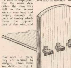
that once in place, they are secured by wedges. Three tusks are shown in Fig. 1, but this is not by any means a strict rule. The number of tusks can be varied according to the width of timber.
