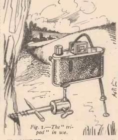
PROVIDED you already posses a ball-socket tripod end, as most photographers do, all that is needed to make the gadget shown in Fig. 1 is a stout woodscrew and a short metal crossbar, which can be made from scrap.
