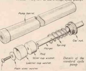
in use on bicycles are ever working at the maximum efficiency, which is a pity because much unnecessary work can be avoided by having an efficient pump.
