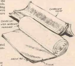
Fig. 9.—Obtaining condenser foil.
