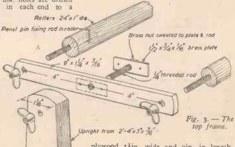
1/16in. holes are drilled about 1in. from the ends carefully positioned to pass through the rod. One inch panel pins driven in from one side of the rail passing through the rods will provide sufficient security.
