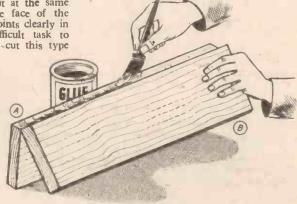
Fig. 5 .- Timber held for gluing.
