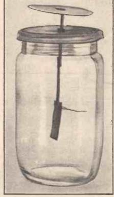
Fig. 8.—Type "B" electroscope.
