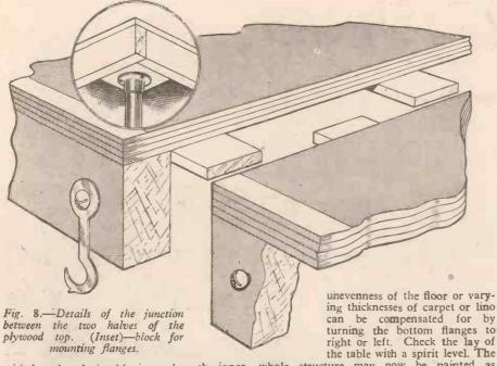
with lengths of 2in. X 1in. and on the inner edge, where they meet, with alternate struts as already explained and shown in Fig. 8. The corners of the 2in. × 1in, framework can well be mitred, but there is no objection to their being butted. At the four corners and at about 3in, from the ends where the table meets in the centre, blocks of 2in. X 2in. wood should be fastened to the frame (see inset, Fig. 8). These serve as supports for the top flanges.
