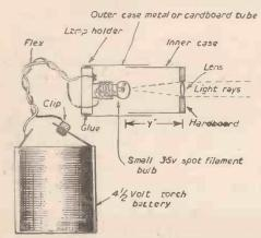
Fig. 32.—Section through the lamp body and connections to battery.
