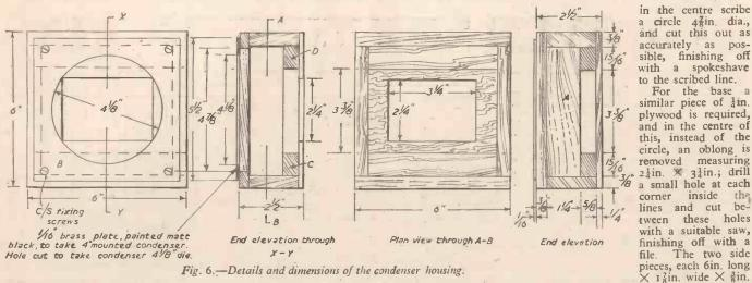
Fig. 6.—Details and dimensions of the condenser housing.
