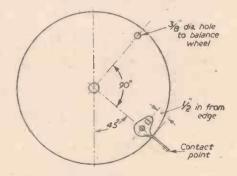
Fig. 3.—Positioning the contact point.
