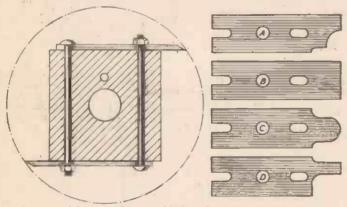
Fig. 15.—A home-made cutter block and cutters. A is a moulding cutter, B is for small rebates, C is for grooving, and D is a fluting cutter. Only one of each is shown, but the cutters must be used in pairs.
