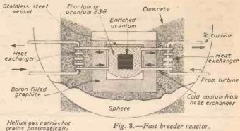
Fig. 8.-Fast breeder reactor. Fig. 9 (Left).—Suspop reactor.
