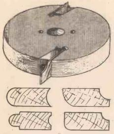
Fig. 14.—A commercial cutter block. The thin cutters are secured by wedging and may be ground to a different profile each end as shown.
