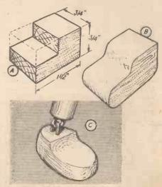
Fig. 11.—Stages in making the foot.
