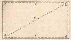
Fig. 6 .- Inserting level pegs inside the area.
