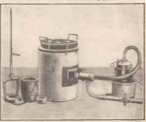
Miniature crucible furnace, fired by gas
