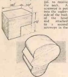
Fig. 12.—Basic shape of the head.
