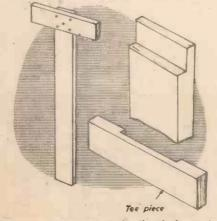
Fig. 3.-Constructional details of the bonirods
