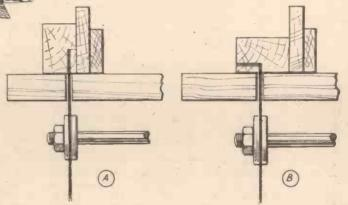
of flooring or match-boards lying about the workshop, and these are suitable for the purpose. In Fig. 11 an 8ft. by 4ft. sheet of hardboard is being sawn down the centre, single handed, with the assistance of grooved strips pinned to the edges, as shown in the inset sketch. A large sheet like this is best cut half-way best cut half-way along the length, then lifted clear of the saw,
