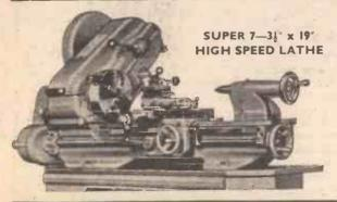
Standard Super 7 accommodates 10" in Gap—7" over Bed and 4½" over Boring Table. Full length 19" between Centres. Advanced Spindle Design—Cone Bearing at Front and Twin Angular Contact Bearings at Rear—14 Spindle Speeds from 25-2150 r.p.m. Clutch Control. Long Boring Table to carry Rear Tool Post, Friction Setting Index Dials. Ejector Type Tailstock, etc.
