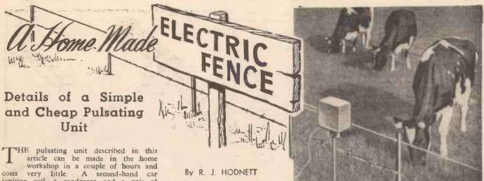
article can be made in this article can be made in the home workshop in a couple of hours and costs very little. A second-hand car ignition coil, a condenser and a pair of contact points are the only items the constructor will have to purchase. No springs are used either on the armature or on the balance-wheel as the unit operates in a vertical position and depends on gravity for its action. The completed pulsator is shown in Fig. 1.
