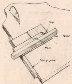
Fig. 16.—The sliding jig used for accurate crosscutting.
