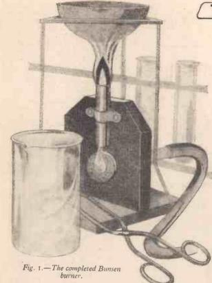
BUNSEN burner is a valuable piece of apparatus to the home chemist or to anyone wishing to temper small
