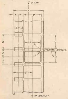
Fig. 1.—Principal dimensions of 8 mm. film.
