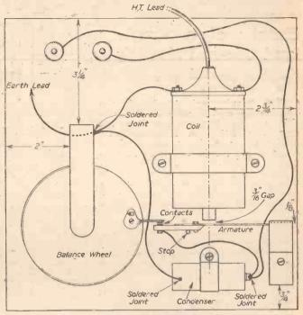
Fig. 5 .- Position of components and wiring.
