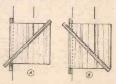
Fig. 18.—Similar sliding jigs, but with the fence, at 45 deg are used for sawing mitres.
