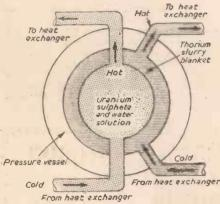
Fig. 2.—Homogeneous power reactor.
