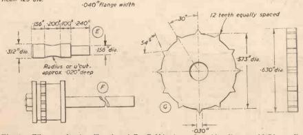
Fig. 6.—Film sprocket (2 off). A and B—Bobbin (turn from §in. diameter M.S.), I off each per sprocket. C—Disc (turn from 41/64in. diameter M.S.), I per sprocket. D—Spindle (turn from standard axle), I per sprocket. E—Pad (turn from 5/16in. diameter M.S.), 2 per sprocket. F—Sprocket assembled on spindle. G—Enlarged view of toothed disc.
