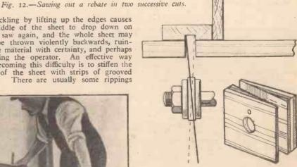
Fig. 13.—Cutting grooves with a "wobble" saw. The tapered collars are used in pairs, one on either side of the saw.
