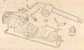
Only 16in. long, the Emco-Unimat is capable of several standard workshop practices to highly critical limits. The basic tool will buff, turn, polish, drill, grind and mill, and a full range of extra equipment vastly increases the scope of the tool.
