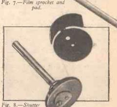
removed showing 8 mm. c.a m (.432in.) spigoted to 9.5 mm. cam wheel.
