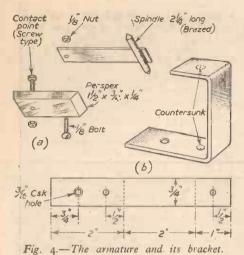
to one side if necessary. Tighten up, the 3/16in. bolt and nut clamping the contactpoint in position and also the screw attaching the armature bracket to the baseboard.
