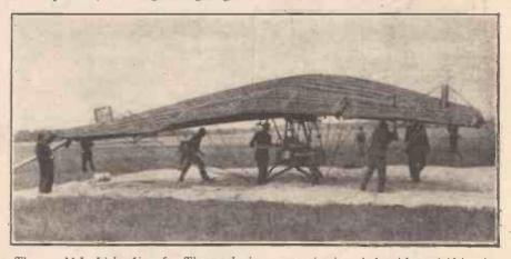
The new M.L. Light Aircraft. The novel wing construction is entirely without rigid bracing and is an inflated fabric envelope, in which pressure is maintained to provide a stiff aerodynamic surface. The 'plane, with wing collapsed, is towable behind a private car.
