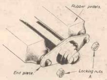
Fig. 3.—Removing pedal rubbers.
