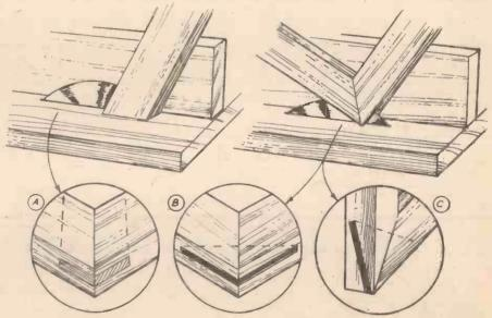
Fig. 20.—Mitred joints may be strengthened by grooving and fitting glued "keys" of veneer cr plywood.
