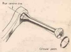
Fig. 4.—A bent spindle tip describes à circular path.
