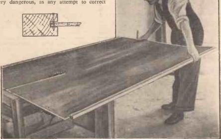
Fig. 11.—Large panels of plywood or hardboard can be cut if the edges are stiffened with grooved strips pinned on to prevent buckling.
