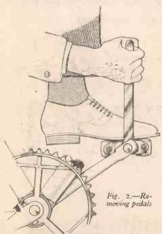
provided by means of a threaded cone, which is locked in position with a keyed washer and a nut. The spindle shell, ball cups and pedal frames are all formed in one spiece and should not be dismantled. A hub cap protects the bearings against the incursion of dust and rain, etc.
