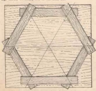
Fig. 19.—A useful method of cutting mitres.
