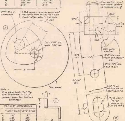
Fig. 4.—A—The cam, made from 17 b.w.g. (.058in.) M.S. B—The follower, made from 17 s.w.g. (.056in.) M.S. C—Plan view of the claw (18 s.w.g. (.048in.) M.S.).
