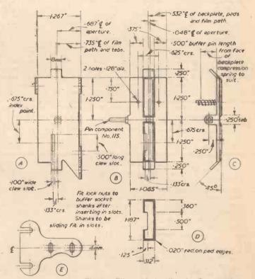
Fig. 2.—Film guide (1 off). A—Gate bracket, made from 19 s.w.g. (.040in.) brass. B and C—Backplate (with pads fitted) made from 19 s.w.g. brass. D—Lower pad, made from 20 s.w.g. (.036in.) brass. E—Buffer bracket, made from 14 s.w.g. (.080in.) brass.
