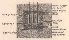
Fig. 6.—Heavy water reactor.
