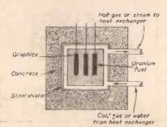
Fig. 4.—Graphite moderated reactor.
