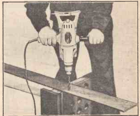
(Right)—The Wolf \frac{1}{2} in. capacity two-speed portable drill.
