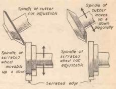
Fig. 7.—This arrangement probably gives a slight undercutting effect to neaten the cut edge of the lid.
