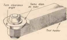
Fig. 3.—A tool holder which a lathe user can make for turning profiles similar to that needed for the machining of these grooves in the rolls.
