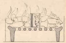
Fig. 9—Tin of slack coal placed in fire to be coked and burnt.
