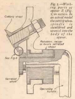
can (ready for cutting to start) at the end of its stroke. The fact that in this and other openers the axis of the cutting wheel is set out of parallel with that of the serrated wheel in the horizontal plane, as well as in the vertical plane, is being ignored
