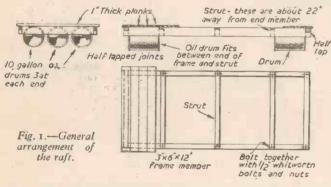
As the raft is afloat for several months and is not likely to receive any attention during that period, and as the timber is very little use for other articles after such a spell in the sea, there is no need to plane the surfaces. Provided any old nails are pulled out and any broken strips of wood likely to cause injury are removed there is no need to prepare the timber, and one can go ahead with the jointing prior to bolting the framework together.
