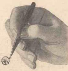
Fig. 6.—The miniature power plant built into the balance wheel of the electric watch.
