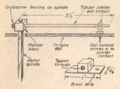
Fig. 6.—The pointer and pointer contacts.
