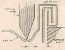
3.—Enlargement of detail inside circle in Fig. 2. The gap between cutting wheel and servated wheel is so wide that the can lid bends instead of shearing.
