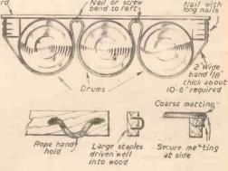
Fig. 5.-Fitting the drums, the rope handholds
