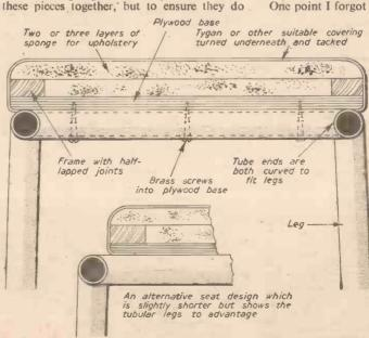
Fig. 5.—A cross-section through the seat illustrating the method used for attaching it to the frame.
