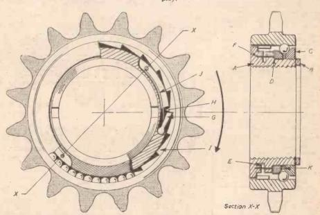
Fig. 2.—A freewheel cut away to show assembly and a sectional view.
