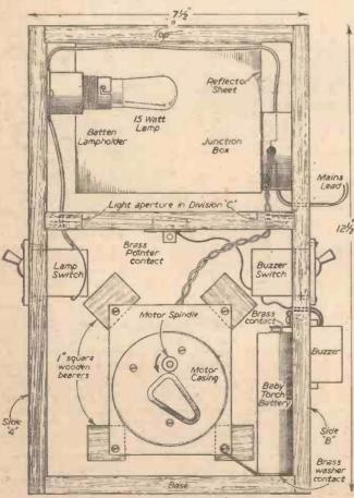
Fig. 1.—General arrangement of Safetigat and Timer
