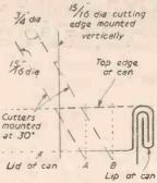
Fig. 4. — showing how the distance of the cutting edge from the serrated wheel, when working round corner of lin. radius can be reduced by inclining the cutter as at A and by reducing the dia-
