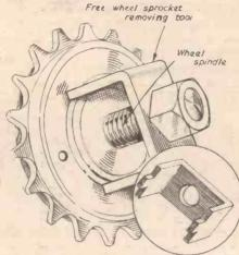
Fig. 1.- Freewheel removal tool (inset) and how it is used.
