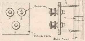
Fig. 4.—The terminal panel. Distance pieces are not shown.
