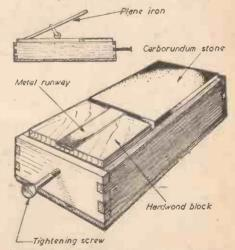
Extending the carborundum stone to increase its efficiency and lengthen its life.
