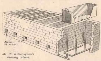
How can I arrange the steam piping to the "steaming cabinet"? I do not want to get the L.P. and H.P. steam systems mixed, as the former is exhaust steam from the steam engine (back pressure steam) and the latter is direct steam from the boiler.
