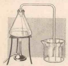
Fig. 1.—Apparatus for making hydrochloric acid.
