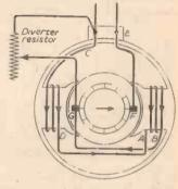
Fig. 3 (Left).—Connections a compound motor.
