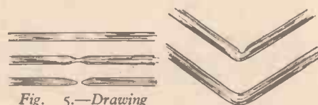
Fig. 6.—Correctly and incorrectly formed bends.
