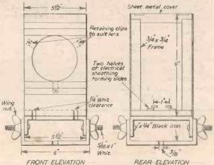
Fig. 2.—Front and rear elevations.
