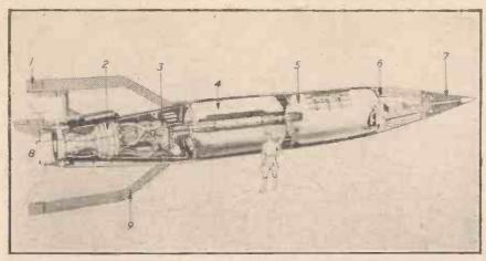
Fig. 8.—A sectional view of the V.2. 1. Four external control vanes; 2. Combustion chamber and venturi; 3. Turbine and pump assembly; 4. Liquid-oxygen tank; 5. Alcohol tank; 6. Control compartment; 7. War-head; 8. Four internal control vanes; 9. Four stabilising fins.
