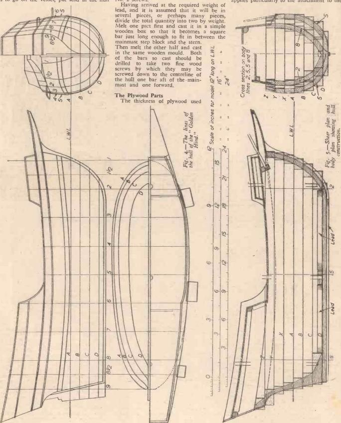
hull. It could be glued, but screws would still be needed to pull the joints up tight, and as it may be convenient at some time to take some part away for repair or to obtain access to the inside of the hull it would be better to leave the joints dry. The only exception is the forecastle, but casein glue would be unsuitable for these small pieces and the use of celluloid cement is suggested here, of the kind which is used in model aeroplane construction:
