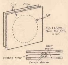
Fig. 2 .- Cementing the filter between two cover glasses.
