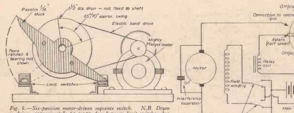
is driven approximately 65 to 70 deg. between limit switches, but the six-position ratchet (behind) only moves the shaft in 60 deg. steps.
