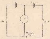
Fig. 1.—Basic two-battery mark/space steering circuit with limit switches (L.S.).
