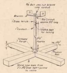
Fig. 4.—The stand and mounting bracket.
