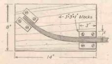
Fig. 2.—The bending fixture.
