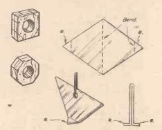
Fig. 3.—Construction of the tinplate triangle and the wooden washers.
