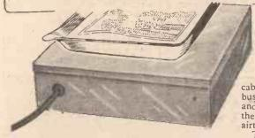
THE dishwarmer described is used for print dish and developing tank solutions. The thermostat keeps the solution temperature to within half a degree of what is required. Any temperature setting can be obtained by altering the thermostat adjusting screw.
