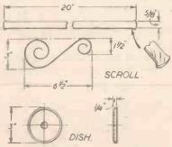
Fig. 2.—Dimensioned views of all the parts.
