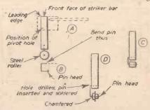
Fig. 3.—Modifications to the striker wheel and striker bar.
