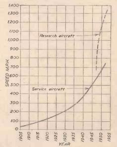
Fig. 1.—Increase in the maximum speed of aircraft during the first half-century of flight.
