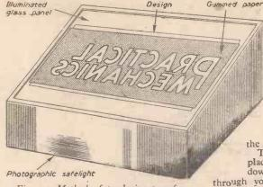
Fig. 1.-Method of producing transfers.
