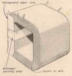
Fig. 2.—Fitting protection strips.
