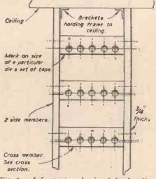
Fig. 3.—A front view showing holes for dies.
