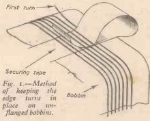
of one length being soldered to the beginning of the next, the joint being a "side-byside" one and lying flat on one of the bobbin faces; adjacent turns to the joint should be spaced away by one wire diameter.
