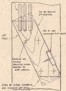
Fig. 2.—A side elevation showing constructional details.
