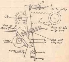
the uprights (B and Fig. 6.- The motor and countershaft assembly.
