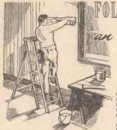
THE folding steps shown in Figs. I and 2 are light and easily made and are preferably constructed in hardwood such as birch. If made from yellow deal or other softwood, the dimensions for the finished wood thickness should be slightly vincreased.
