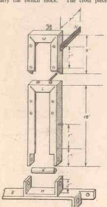
Fig. 5.—General assembly of motor countershaft frames.
