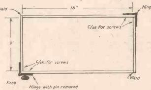
Fig. 1.—Constructional details of the casting frame.
