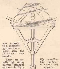
around the periphery of a revolving plate—each mirror being responsible for one film frame in each sequence of eight. Because the mirrors are rotating with the mirror plate they have to be made to tilt in two different ways—one tipping forward to take care of the downward movement of the film, the other swinging round to take care of the rotation of the plate.
