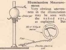
Fig. 5.—Measuring strength and evenness of illumination.
