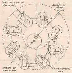
Fig. 8.—The position of the tripod roller at successive instants.
