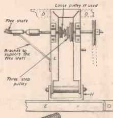
Fig. 9 (above) .- The countershaft line-up
