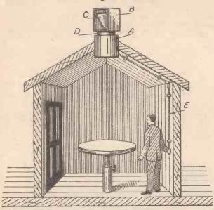
Fig. 1.— The interior of a camera obscura.
