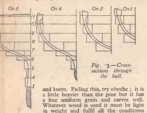
named. Have all the planks cut, thicknessed and surface planed so that they are all, except two, a uniform thickness of exactly rin. Any discrepancy will result either in the model being above its regulation depth or it will have a smaller displacement.
