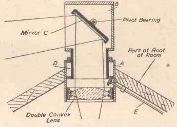
Fig. 2.—Section through the lens and reflecting mirror.
