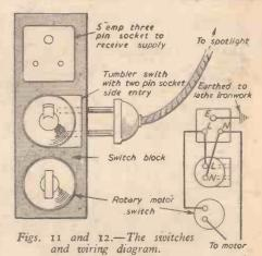
two-pin socket. The motor switch is of the rotary type to avoid confusion. The lamp can be mounted on D and can be of any adjustable type. A wiring diagram is given in Fig. 12. Make sure that the switches are connected in the "live" side. If in any doubt do not run any risks, call in an expert. A radio and TV suppressor should be fitted to the motor.
