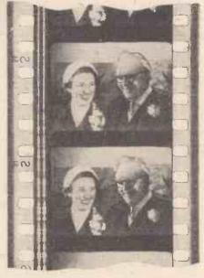
Fig. 1.—A strip of commercial 35 mm. cinema film, showing sound track at side.
