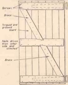
Fig. 4.—Constructional details of the doors.
