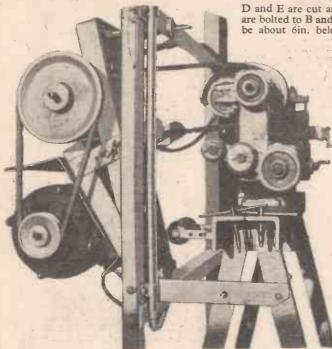
A view-from the left of the lathe stand. Note shield round motor.
