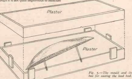
with liquid plaster of paris and the fin pattern, well greased, is embedded in this up to its centre line all around. When the plaster
