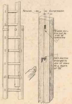
Fig. 4 (Left).—A perspective view of the completed ladder.
