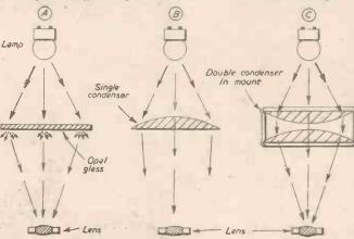
Fig. 2.—Diffused and condenser lighting.
