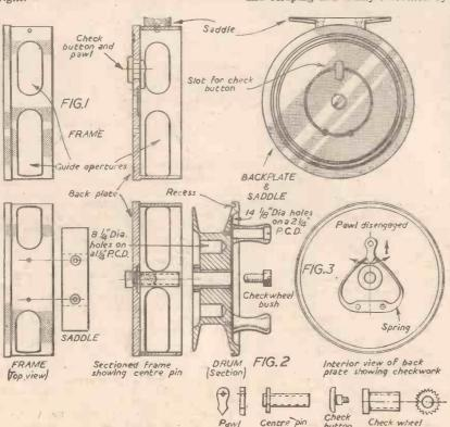
Figs. 1, 2 and 3.—Details and dimensions of the component parts of the reel.
