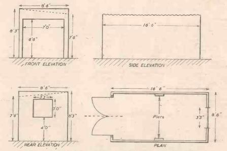
Fig. 1.—Side, front and rear elevations and plan view, giving chief dimensions.
