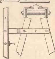
Fig. 3.--An end view of the lathe bed (A) and the supports (G).
