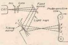
Fig. 3.—A simplified picture showing the arrangement of fixed and tilting mirrors in the Mechau camera.
