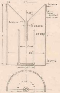
Constructional details of a rain-gauge.
