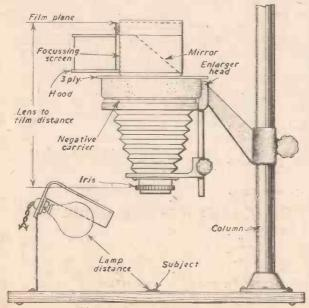
Fig. 1.- Set-up with reflex camera.
