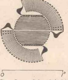
Fig. 4.—Four-gauge diaphragm developed in conjunction with the Admiralty Research Laboratory.
