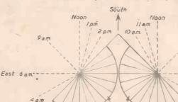
15° intervals Fig. 2.-The use of two half cylinders enables sun to be recorded from sunrise to sunset on a June day. Note marking of 15 deg. hour lines on blocks holding recording papers.
