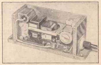
Very sensitive in- Fig. 2 .- View of the de Havilland moving coil pick-up with cover removed. Note the compactness of this instrument.
