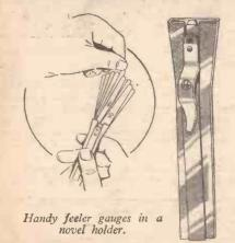
are not easily damaged as the sets are not of the fan type, but if they do become bent or otherwise spoiled, they can be readily withdrawn for replacement.
