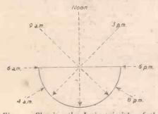
Fig. 1.—Showing the basic principle of the sunshine recorder—a half cylindrical pinhole camera. Note that a single cylinder will record somewhat less than 12 hours sunshine only.
