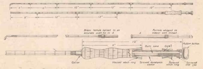
Fig. 1.—The completed rod, showing spacing of the rings, the joint ferrules and the handle construction.
