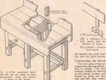
with the top cut away to show construction. Only one drawer is shown in this sketch.
