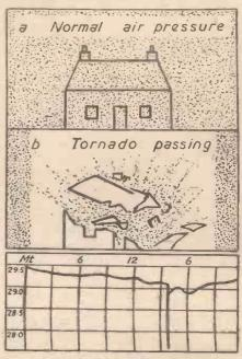
Fig. 11 (top).—The explosive effects. (Bottom) Typical barogram of a tornado.
