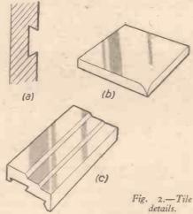
there are not more than about four of these tiles used on the fireplace. In the design showh in Fig. I the three-round-edge tiles used at the top of the surround were made up from halves of two adjacent-round-edge tiles.
