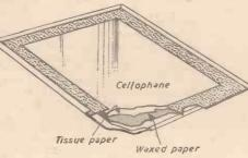
Fig. 3.—Assembling the writing tablet.
