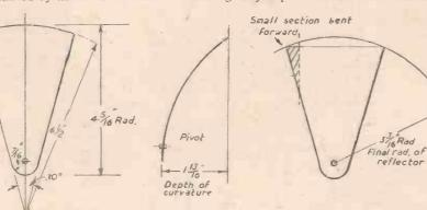
Fig. 2.- The development of the reflector segments.
