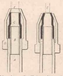
Scheme for an adjustable jet, working on the same principle as an adjustable hand drill or brace.
