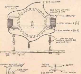
Fig. 2.-Constructional details and dimensions of the motor.
