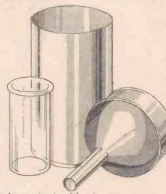
A perspective view of the rain-gauge components
