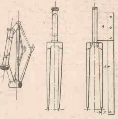
Fig. 6 (left).—Shows a twisted frame. Fig. 7 (middle) forks set sideways; and Fig. 8 (right) checking forks for truth.
