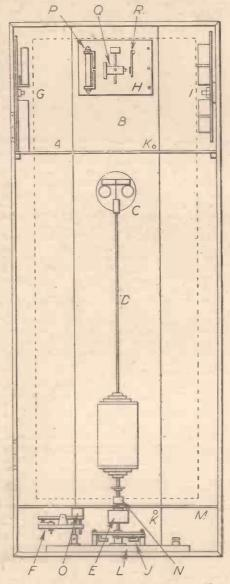
Fig. 1.—Lay-out and general principle. Key: A—Movement shelf; B—Backboard; C— Suspension; D—Pendulum; E—Motor Coil; F—Magnetic switch; G—Power unit; H— Escapement; I—Reserve batteries; J—Advance and retard switch arm in normal position; K—Hole in backboard through which 4 leads pass; L—Motor platform; M—Motor cover; N—Armature; O—Permanent magnet; P— Escapement coil; Q—Escapement armature; R—Escapement contact.
