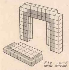
concrete is needed to bond them together and to provide a solid backing for the tiled front. Some people have the impression that a tiled fireplace is made by fixing the tiles to a slab of concrete with tile cement. With the older type of fireplace this might have been done, since the building of them was more in the nature of a wall-tiling job. The modern tiled surround is made by laying out the tiles in the form of a mould and then filling in with concrete.
