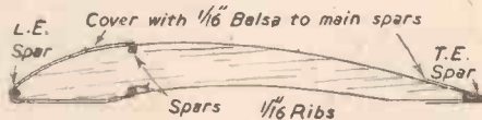
Fig. 11.—Stiffening up the wing by covering L.E. and T.E. with sheet balsa.
