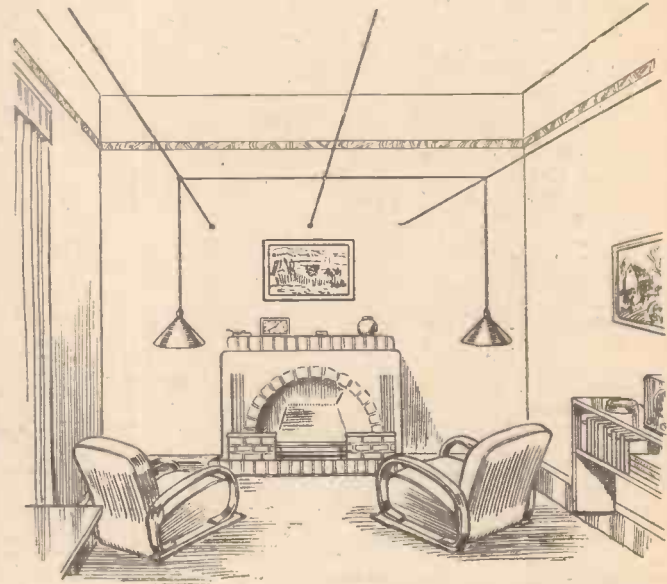
Fig. 1.—Arrangement of lights in living-room. Separately switched 12- or 18-watt bulbs, suspended by flex from bare 7/22 aerial wire stretched from walls at a height of about 9ft.
