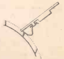
Fig. 3.—The free end of the damping spring should be as close as possible to the point of the key.
