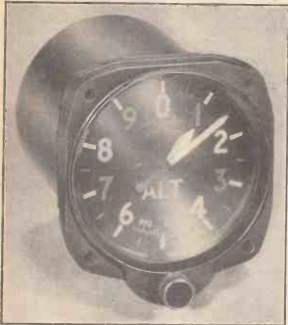
An ex-Government altimeter with millibar scale visible through window in dial.
