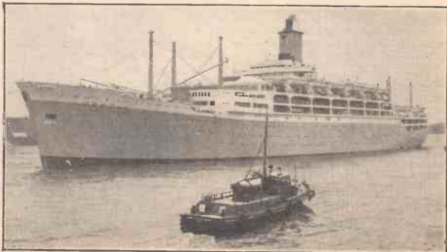
The new Orient liner "Orsova," 29,000 tons, leaving Tilbury recently on her maiden voyage to Australia. Unusual features of the liner are the absence of conventional masts and the extension on top of the funnel designed to keep smoke well clear of the decks.
