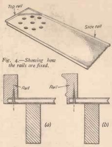
Fig. 5.—Sections of the side rails.
