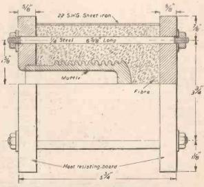
Fig. 2.—A side clevation in part section of a 200-watt electric furnace.
