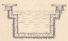
Fig. 5.-Method of arranging dwarf walls surmounted by projecting coping slabs.
