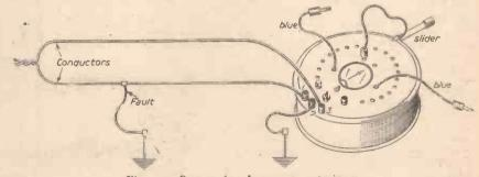
Fig. 9 .- Set-up for loop test experiment.
