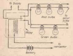
Fig. 1.-Relay circuit for changing colours.
