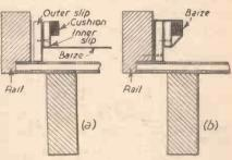
Fig. 7.—Sections of slips and cushions.
