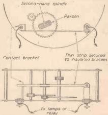
Fig. 3.—How the contacts are actuated.
