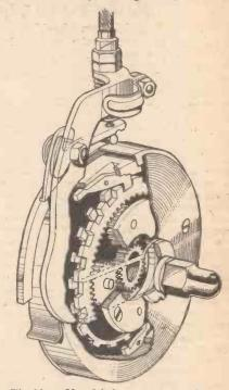
The Novo-Vaxel hub type two-speed gear.
