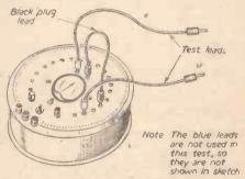
Fig. 11.—Using the instrument as a D.C. voltmeter.
