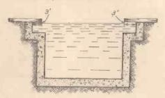
Fig. 4.—Using concrete slabs to cover the edges of the pool walls.
