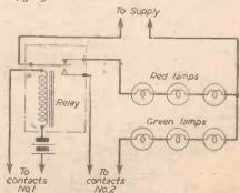
Fig. 4.—Change-over and flashing circuit.
