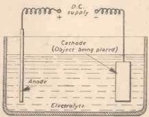
Fig. 3.-Diagram of connections to plating
