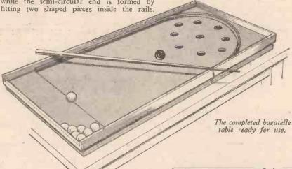
Cushion slips and rubber cushions are fitted around the rails and the semi-circular end, and pegging or scoring holes for 100 up are drilled in the upper edges of the rails.
