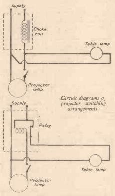
plugs into a wall switch plug, rather as a two-way adaptor does. It has two two-pin sockets—one for the projector and one for a table lamp. The current is switched on, lighting the table lamp, and when the projector is switched on (it has its own switch built in) then the table lamp goes out; when the projector is switched off, on comes the table lamp.
