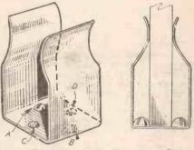
Fig. 5.—How to make the glass cip for Fig. 4. C and D are soldered ends of the contacting suites.
