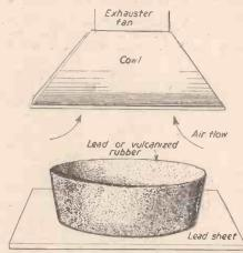
Fig. 2.—Simple equipment for etching. The fan can be replaced with a chimney stove pipe if the up-draught is sufficiently strong.
