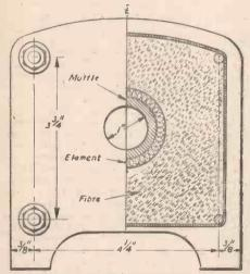
Fig. I .- An end elevation in part section of a 200-watt electric furnace.
