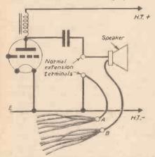
Fig. 1.—How to arrange the output circuit for radio games.
