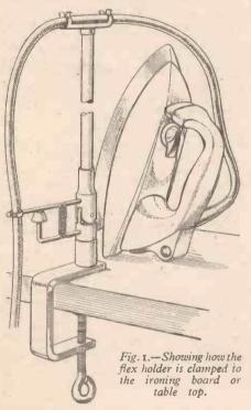
hampered use of the iron over the whole of the table area, following the movement of the iron in all directions, and gathering back the flex when the iron is returned to its stand position.
