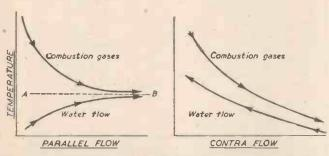
Fig. 2.—Parallel flow gives a low water temperature and high gas temperature. AB represents the theoretical limit of both. Contra-flow gives higher possible water temperature and lower gas temperature, hence higher efficiency.
