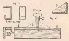
Figs. 3 and 4.—Details of bath clamp, and side elevation of base.
