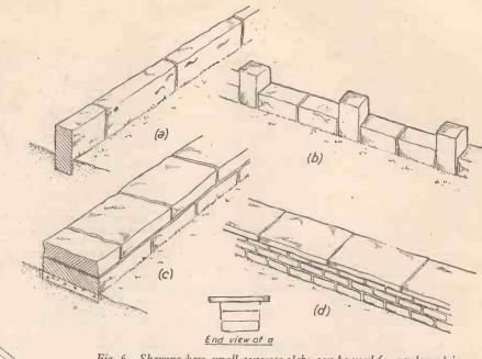
Fig. 6. Showing how small concrete slabs can be used for garden edgings.
