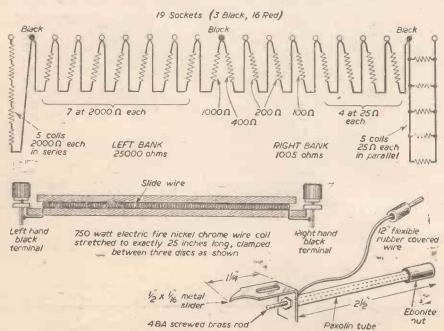
Fig. 2.—Arrangement of resistances and details of slide wire and slider.
