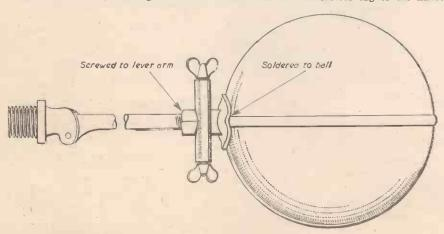
Fig. 1.-Showing how the fitment is attached to the ball valve and the end of lever arm.
