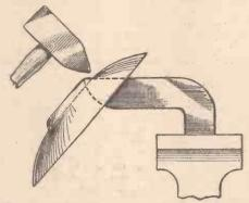
Fig. 1-Forming a step on the first guide-line.
