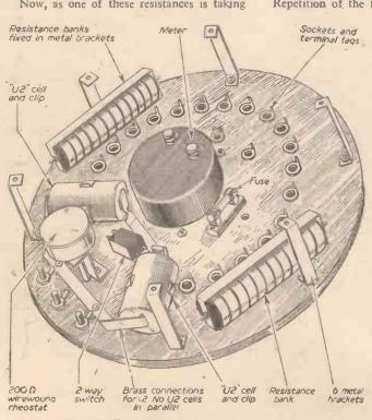
Fig. 6.—Underside view of the panel, minus the winding, showing the layout of components.
