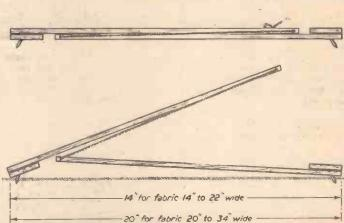
Fig. 14. Details of tenterhooks for fabric up to 15 in. wide.
