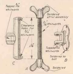
Fig. 2.- Details of the ball-valve adjustment device.
