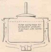
Fig. 4.—Sectional view showing cylindrical casing.
