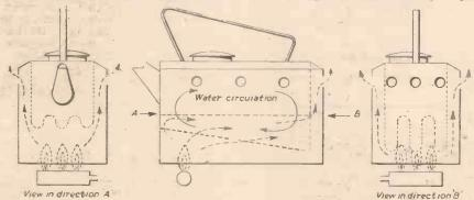
Fig. 7.—A design for a kettle giving increased heating surface area, completed combustion, contra-flow and stimulated circulation.
