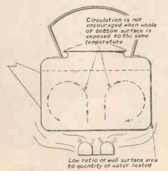
Fig. 3.—The conventional kettle.
