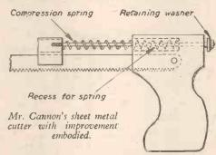
may I offer the following suggested improvement? By dispensing with the coil spring at the top of the body, and substituting a compression spring round the 4 B.A. rod, as in accompanying sketch, and counterbored into the body, the tool is somewhat neater and, mechanically, the line of action of the spring is correct, instead of tending to cause the rod to bind on the side of the hole.—A. S. FRASER (Tottenham).
