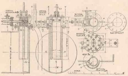
Fig. 5.—Details of the cylinder, valve and piston.
