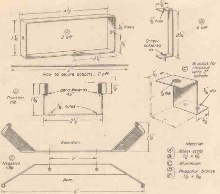
Fig. 5 .- Details of the metal brackets and chps.
