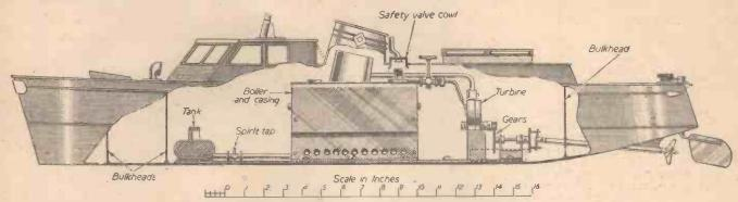
Fig. 3.—Showing the location of the turbine power unit in a model boat.
