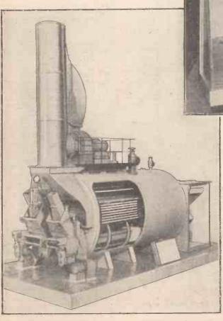
Fig. 3.—A model of Edwin Danks patent high-velocity economic-type boiler, to a scale of  $1\frac{1}{2}$  in to 1 ft. Part of the boiler shell is cut away to reveal the interior.
