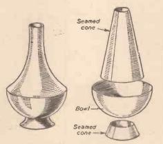
Fig. 3.-Fabricated cone shapes.
