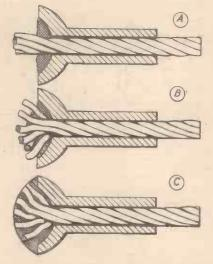
Fig. 2.—A: cable is soldered into the nipple: B: the end is splayed: C: the whole is fixed and sealed with a blob of solder.
