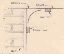
How slipper and nib rails are used as guides.
