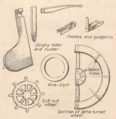
Figs. 4 and 5.—Dinghy tiller and details of steering wheels.
