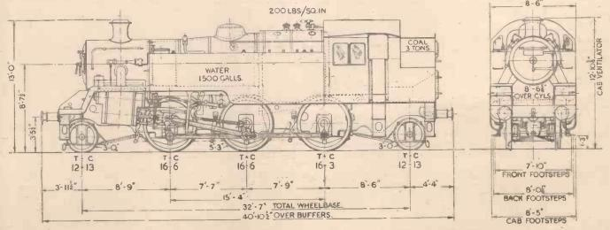
Side and front elevations of the new locomotive, giving some of the leading dimensions.
