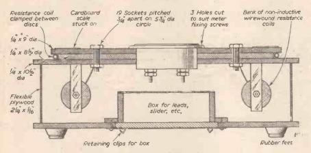
Fig. 4.—Sectional view of the testing set.
