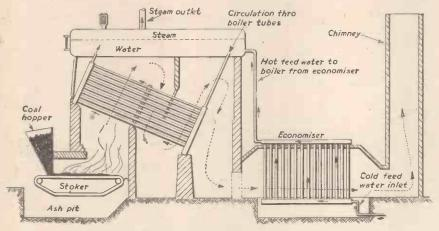
Fig. 1.—Sectional diagram of an industrial water-tube boiler.
