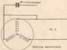
Connections for converting a three-phase motor to single phase.
