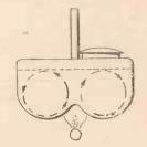
therefore pass through the mass of water as well as round it. A section of the additional outer casing is cut away to allow the gases from the internal tubes to pass directly out to atmosphere.
