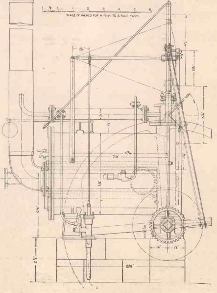
Fig. 2.—Side elevation of the Trevithick model.
