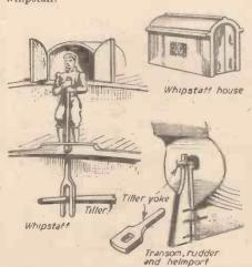
Figs. 2 and 3.—Details of the whipstaff, tiller yoke and helmport.
