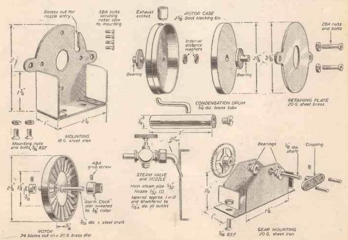
Fig. 1.—Details of the turbine and gear-case components.
