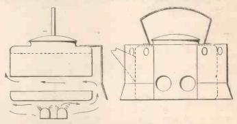
Fig. 5.—Two views of a conventional kettle with the addition of internal tubes and outer casing.
