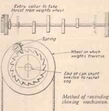
which the weights are suspended) the wheel on which a rachet is fixed revolves freely on the camshaft. Engaging the ratchet is a cog-wheel which is sweated to the camshaft end.
