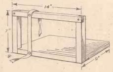
Fig. 1.—Sewing frame with one tape pinned in position.
