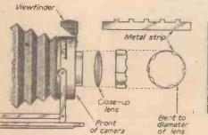
Fig. 1.-A push-on holder for close-up lens Fig. 2.-A simple fitment for bax cameras made from metal strip.
