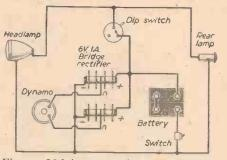
Fig. 2.-Lighting system for a motor-assisted bicycle.
