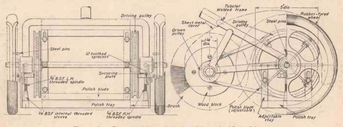
The wheels and axles could, if necessary, be made up from old pram wheels keyed to the axle. The vee-pulleys, belts, ratchet gears and bearings are best purchased. Polish
