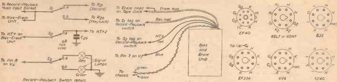
Fig. 5.—Details of wiring of the change-over switch.
