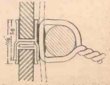
Fig. 5.—An orthodox make-off joint and wire tie.
