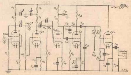
Fig. 1.—Theoretical circuit of the recording section of the equipment.
