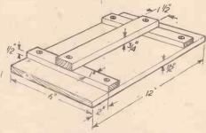
Fig. 3.—Details of a wooden float.
