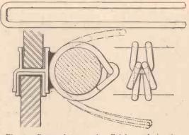
Fig. 6.-Proposed new make-off joint and tie wire.
