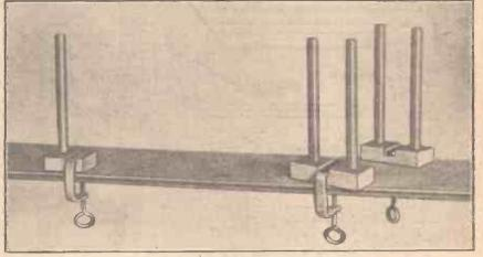
Warping posts, which can be used on a table, shown correctly mounted on a suitable board.
