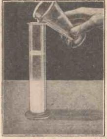
Precipitating pure silver chloride by adding a common salt solution to a solution of silver nitrate. The heavy white insoluble precipitate of silver chloride rapidly sinks to the bottom of the vessel.
