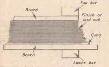
Fig. 5.-Book between boards in clamps, showing the edge partly cut.
