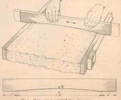
Fig. 2.- Using a screed, and detail giving dimensions.
