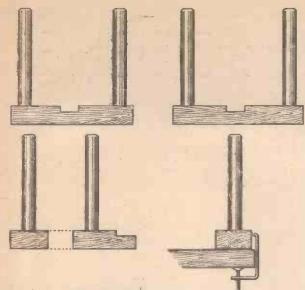
Fig. 13.-Single and double warping posts and clamp.
