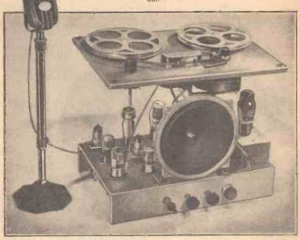
This illustration shows the chassis and tape deck out of the cabinet, and also the microphone.
