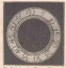
The finished result. The wax-filled seconds circle of a clock dial after its final silvering and lacquering, showing the characteristic contrasts between the black waxed numerals and the matt-silvered background.
