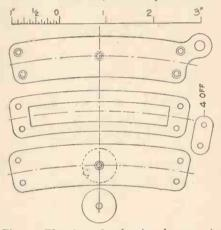
Fig. 9.—The plates for forming the expansion link.
