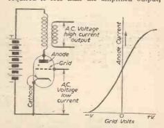
Fig. 8.—Simple triode amplifier.
