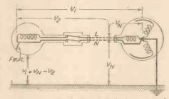
Fig. 2.—Conditions with earth fault on neutral of single-phase apparatus with unearthed metallic sheathing.
