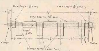
Fig. 8.—Striker shaft and spacers.
