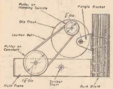
Fig. 5 .- Side view of speed regulator drive.
