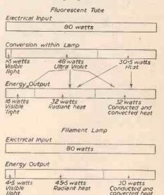
Fig. 3.—The relative efficiency of a fluorescent tube and a filament lamp.
