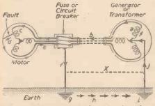
Fig. 1.—Path of earth fault current in a threephase circuit.
