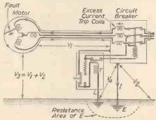
Fig. 6.—Incorrect location of earth electrode for voltage-operated leakage trip.
