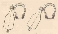
Fig. 2.—Ensure that the pulley wheel is bearing correctly on the side of the tyre.
