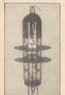
Fig. 18a.—Reflex Klystron CV116. (By courtesy of E.M.I. Research Laboratories, Ltd.)
