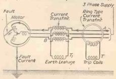
Fig. 7.—Connections of two types of currentoperated earth leakage trips.
