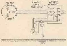
Fig. 5.—Connections of a voltage-operated trip in a three-phase motor circuit.
