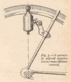
centrated beam, and so on. Sometimes additional refinements are fitted, such as a dimmer or an arrangement incorporating an extra bulb and a battery, which may be brought into operation by the touch of a switch.
