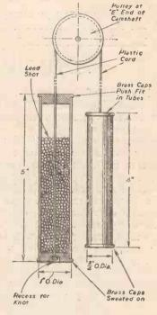
Fig. 4.—Details of weight assembly.
