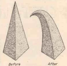
A potter's cone before and after firing to 1,000 deg. C.
