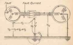
Fig. 4 .- Volt drops in earthing circuit under fault conditions.
