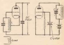
Fig. 11b.—Hartley feedback oscillator circuit.
