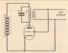
Fig. 10.—A simple valve oscillator circuit.
