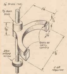
Fig. 6.—Perspective view of camera mount.
