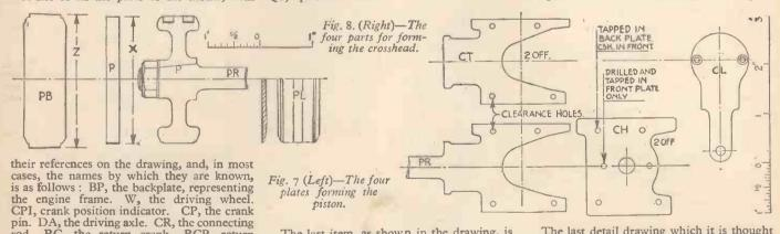
rod. RC, the return crank. RCP, return crank pin. EC, eccentric rod. CH, crosshead.
