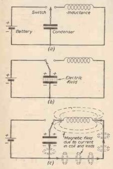
Fig. 5.—Simple oscillatory circuits.
