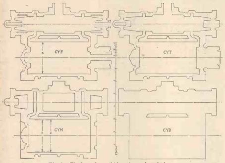
Fig. 6.—The four plates which make up the cylinder.
