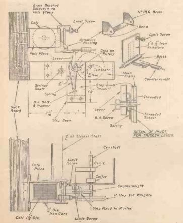
Details of main frame, camshaft Relay The pole-pieces, which form the frame of bearings, and catch. the relay, are made of 1in. by 1/16 in. strip Frame of Hole tor Striker Shatt Holes For Spring Fasteners (See Fig. 1) Rivets Frame Bent on This Line (See Fig.1) For Spring Balt (See Fig. 3) Camshaft Screw Holes For Stop Beam (See Fig. 3)
