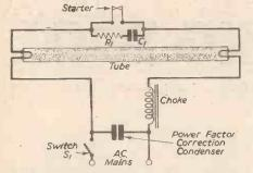
Fig. 1.—Circuit diagram for a single fluorescent Tube.
