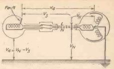
Fig. 3.—Conditions with earth fault on live side of single-phase apparatus with unearthed metallic sheathing.
