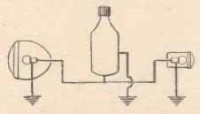
Fig. 1.—The lamps are connected in parallel with the dynamo, and earthing may be carried out either by using the mounting brackets or by connecting the casing of the two lamps to the dynamo casing by means of wires.
