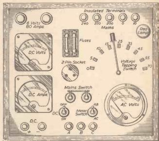
Fig. 1.—The panel of the control box.
