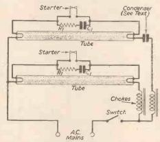
Fig. 2.—Circuit arrangement for twin tubes.
