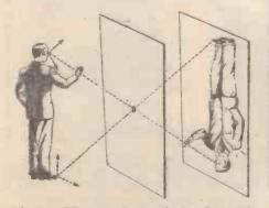
Fig. 1.-Diagram showing image formation.
