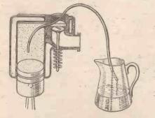
Method of extracting the oil from the cylinder.
