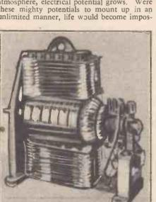
A simple type of dynamo. Essentially this machine is merely a pump for driving electrons through an external circuit.
