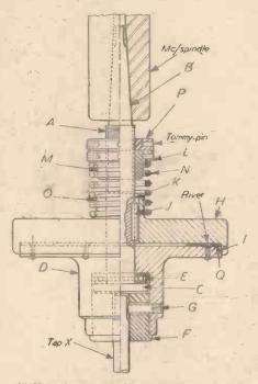
Half-sectional elevation of a friction-driven tap-holder.
