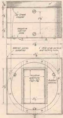
Fig. 1.-Elevation and plan of condenser mount.
