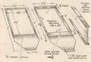
Fig. 3.-Details of negative carrier.
