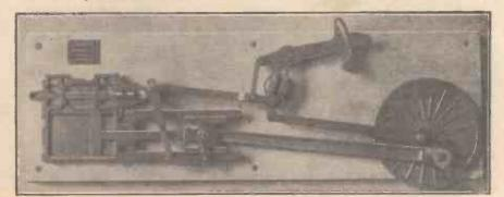
Fig. 4.- A small mass-produced diecast model of the Walschaerts gear.
