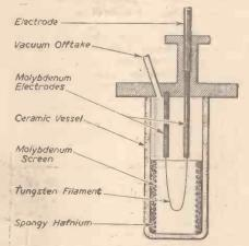
Apparatus for the production of iodide hafnium.
