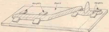
Fig. 4.—Weighting the wing surfaces prevents warping whilst the dope dries. Dope each wing separately, and add weights carefully. Do not apply weights until dope is sufficiently dry to prevent sticking to board.
