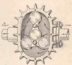
The Roots supercharger for increasing the power of the engine.
