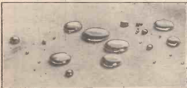
Clean, uncontaminated mercury for barometer use breaks up into globules or "buttons" when spilled on to a level surface.
