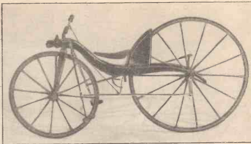
Photograph of the one-eighth scale model of Macmillan's bicycle built by Mr. F. J. Camm. It is to scale in every detail, both as to size and method of construction.
