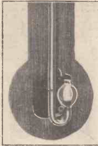
The lower end of a "stick" barometer showing the V-tube whose shorter limb has been formed into a bulbous shape to act as a mercury "cistern."
