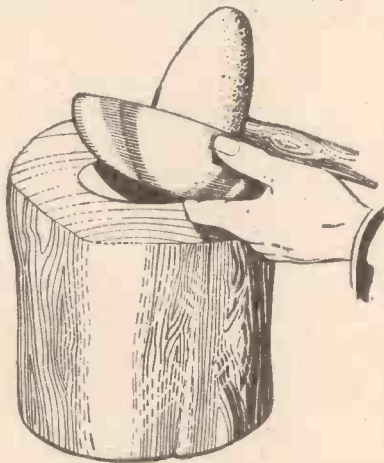
Fig. 1.—Using the bossing mallet on an improvised doming-block.
