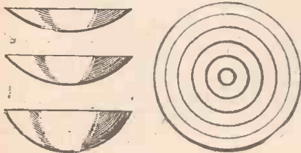
Fig. 2.—Showing how the metal deepens after each course on the doming-block.
