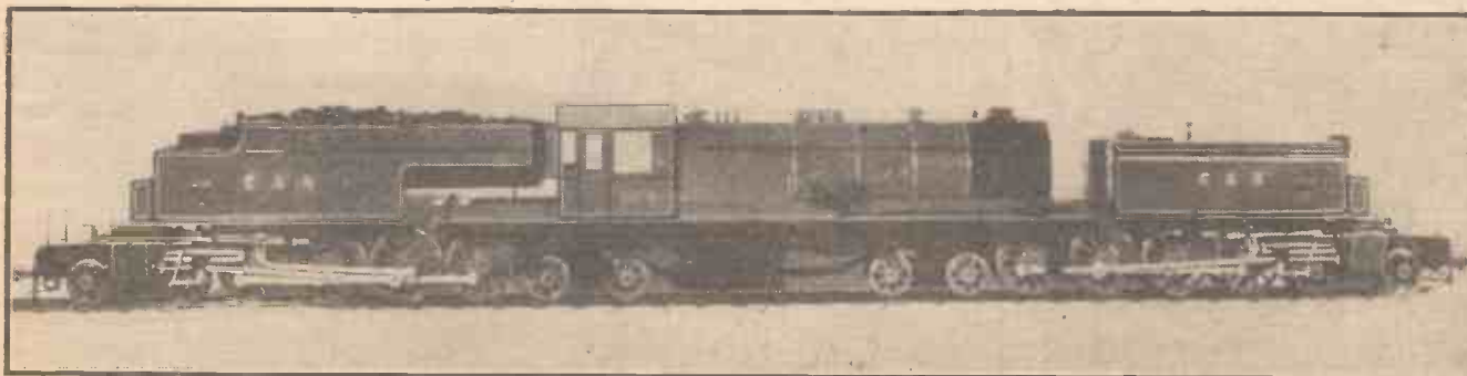
Fig. 4.—A broadside view of an interesting railway model, representing a 4-8-4 + 4-8-4 Beyer Garratt locomotive, to a scale of 1/4 in. to 1ft. This exhibition model has gone to the East African Railways, Nairobi.
