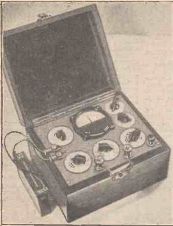
Fig. 1.—The completed resistance bridge, with battery.
