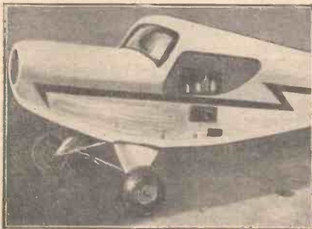
Fig. 20.—A three-valve E.D. "modulated" receiver is seen fitted inside the fuselage of an 8 ft. span model. The receiver is slung by rubber bands to four stout hard-wood dowels built across the cabin.
