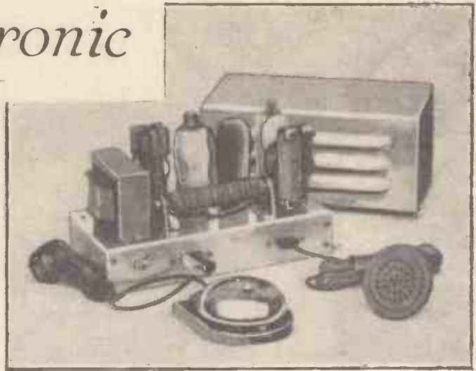
The completed alarm unit with casing removed.
