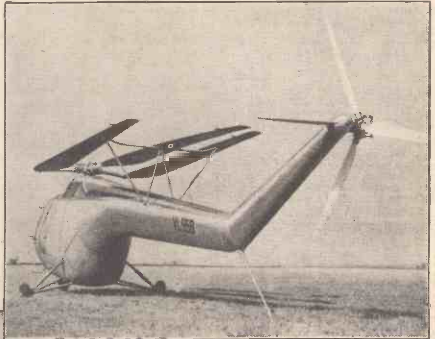
Fig. 4.—The Bristol 171 with rotor blades stowed.
