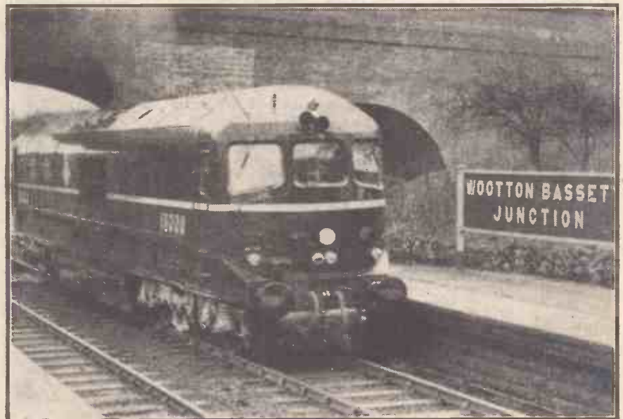
The new gas-turbine locomotive, the first to travel on British Railways, is here seen passing through Wootton Bassett during its first main-line trial. Rated at 2,500 h.p., it reached a speed of 90 miles an hour during tests in Switzerland, where it was built.
