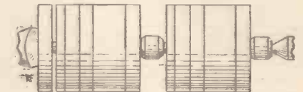
Fig. 96.—How knobs are roughed out previous to turning.
