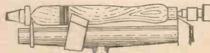
Fig. 48.—Turning a tool handle: the ferrule is slipped over the tailstop centre.
