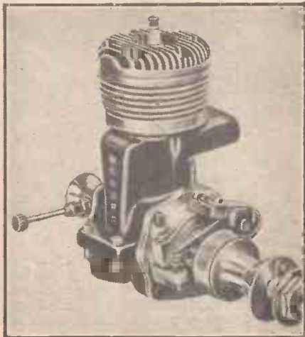
Fig. 17.—The high performance racing Nordec 10 c.c. engine is available in glow-plug ignition or spark ignition form. It is noted for great power at high revolutions and has gained a British record control-line speed of 95.3 m.p.h. Fitted with two piston rings and two ball bearings.
