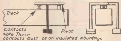
Fig. 3.—Details of the switch S2. Switch S1, at the other end of the track, is of similar construction, but the bevelled edge will slope in the opposite direction.
