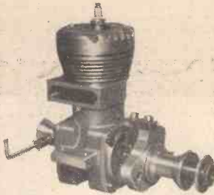
Fig. 15.—The Rowell 60 is a true racing engine on American well-tried lines having a very high performance. This 10 c.c. petrol engine has been officially timed to do 84.4 m.p.h. in a model car and can be bought as an integral unit with spur gearing and axle complete.
