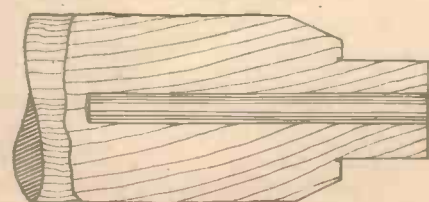
Fig. 49.—Turning a ferrule seating.
