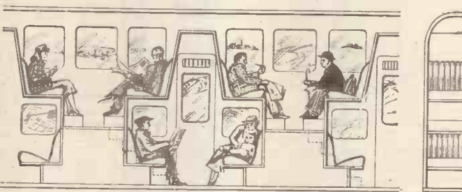
Diagrammatic sketches showing the layout of the upper and lower compartments in the double-decked coach. Note the position of the stairways between the upper and lower decks.
