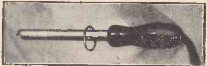
Fig. 5.—The completed igniter. Note the position of the brass ring for hanging up the igniter when not in use.
