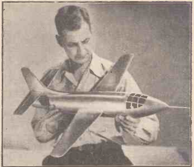
Fig. 10.—This fine example of a control line jet model comes from America, and has an enclosed Dynajet with suitable heat insulation. The air intake is situated inside the open cockpit. (Photo by courtesy of The Dynajet-Aerodynamic Co., Dayton Municipal Airport, Vandalia, Ohio, U.S.A.)
