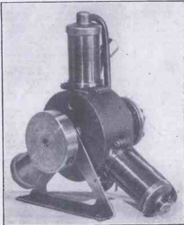
Three-quarter front view of the completed flash steam engine with mounting bracket. A small flywheel has been fitted for test purposes.
