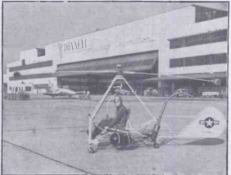
A side view of the tiny aircraft showing the small ram-jet units at the tips of the rotor blades. Weighing only 310 lb., this world's first ram-jet helicopter is capable of a forward speed of fifty miles per hour.
