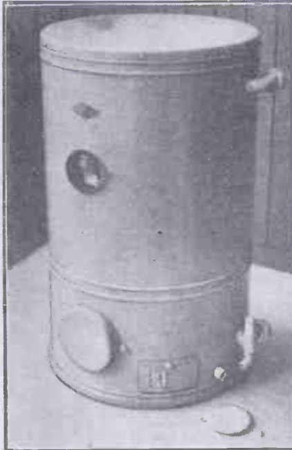
Fig. 16.—Dual water heater (Sadia) of 20 gallons capacity, having two sets of elements. One near the top (cover removed), which provides 6.7 gallons of hot water, and one in base which is controlled by foot switch. This is used when large quantities are required, viz., for a bath.
