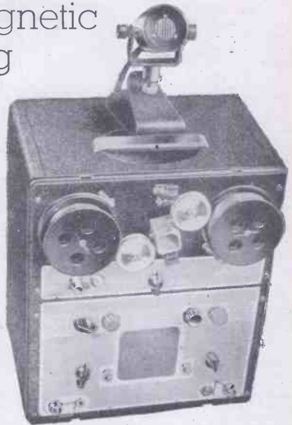
The new British wire recorder, the Model "A" Boosey & Hawkes unit, intended for speech recording.
