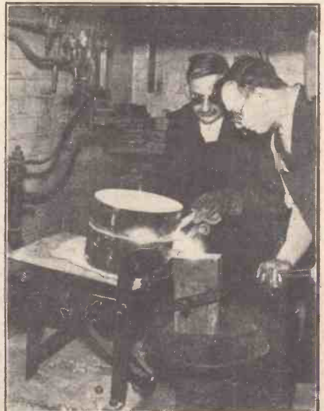
Casting a block of pure platinum in the works of Johnson, Matthey and Co., Ltd.
