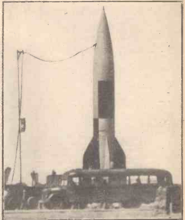
Adapted for the U.S. Army for scientific soundings of the upper atmosphere, this V-2 is seen here being readied for flight at White Sands, New Mexico.
