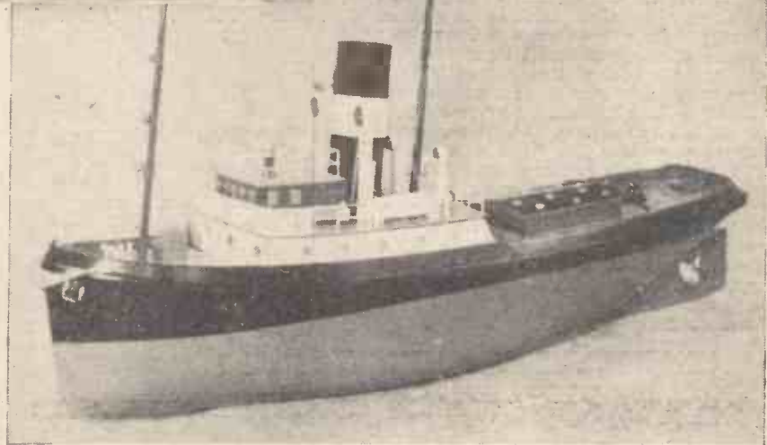
Fig. 2.—Model tugboat by Bassett-Lowke, Ltd. It is 25in. long and is driven by a small electric motor. A dry battery or accumulator provides the current.
