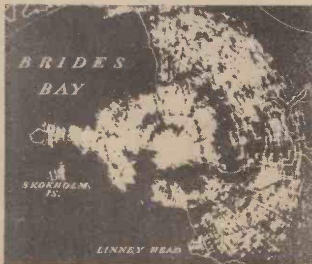
A radar map of the south-west tip of Wales as shown at night on the cathode-ray tube of the H 2 S apparatus on an R.A.F. aircraft.
