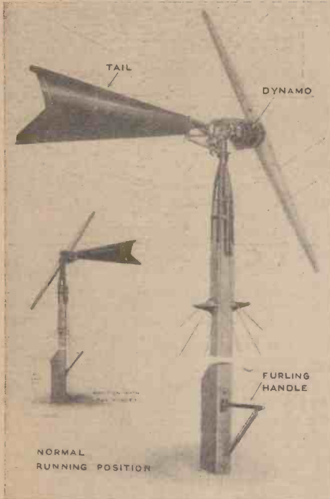
Fig. 1.—The complete wind-driven lighting plant.
